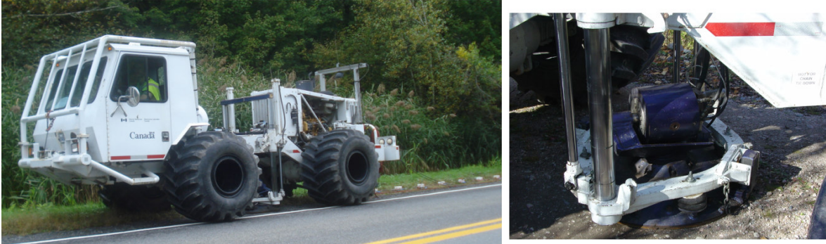
Figure A1-5: Photos of the IVI minibuggy vibratory source. In the photo on the right, the Minivib is being operated in SH-mode (note cylindrical weight above plate is mounted horizontally).
