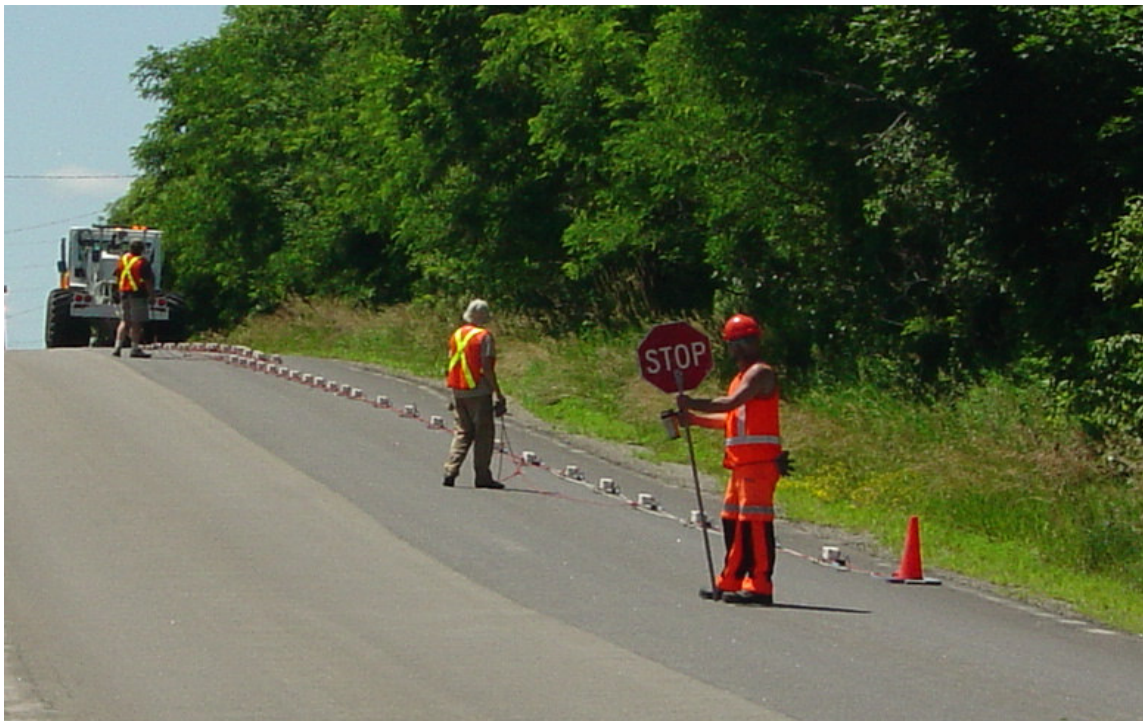
Figure A1-6: Photo of Minivib/landstreamer system in operation on St. John's Sideroad, 2008.
