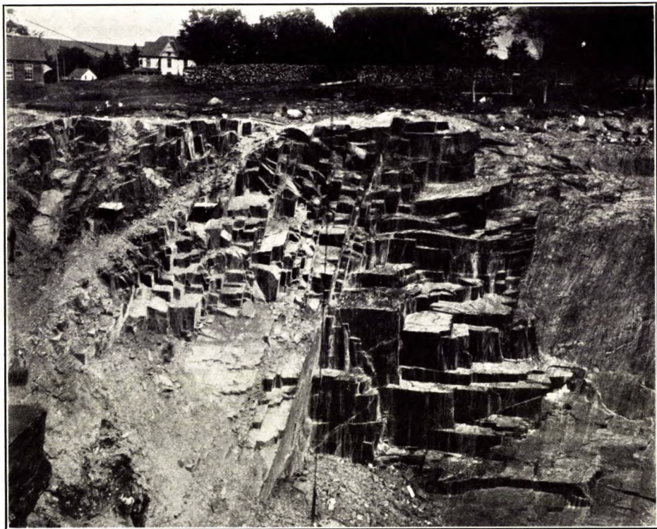
Melbourne slate. Jointing in New Rockland quarry.
