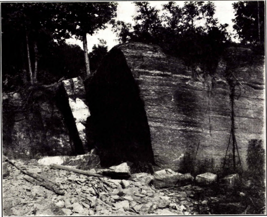
St. Dominique limestone. Quarry showing jointing and weathering, St. Dominique, Que.
