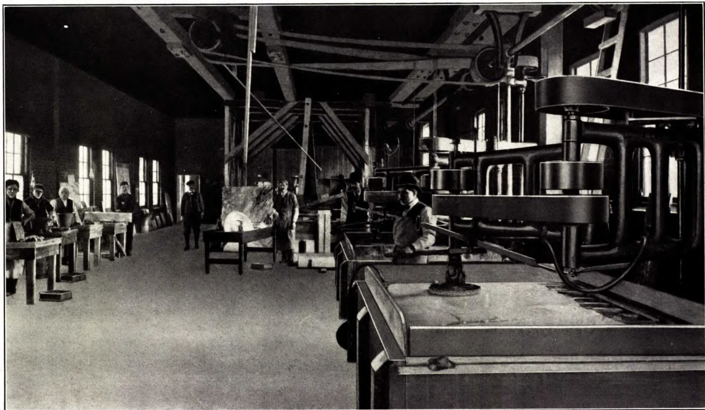
South Stukely marble. Polishing machines in mill of the Dominion Marble Co., Côte St. Paul, Montreal.
