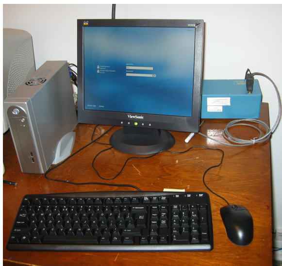
Figure 4. Computer and riometer. A mini-pc (silver box) controls the riometer (blue box) via a RS232 analog to digital converter. The keyboard and mouse are standard size. The monitor is used to view the data collected.
