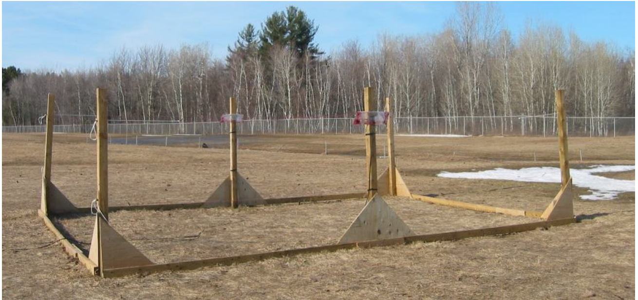
Figure 6. Riometer antenna support for solid rock or frozen ground conditions
