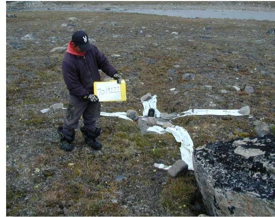
A visible ground location of an existing ground control marker.
