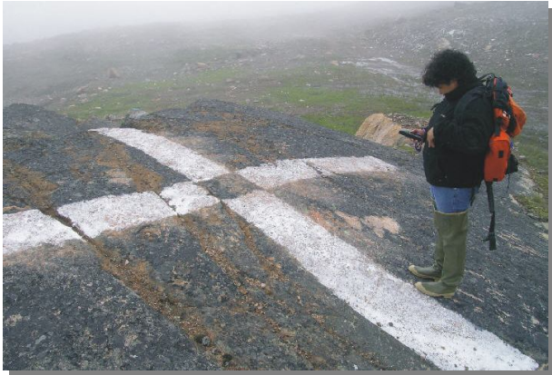
Geodetic Survey ground control points characterized as painted white crosses on the ground.
