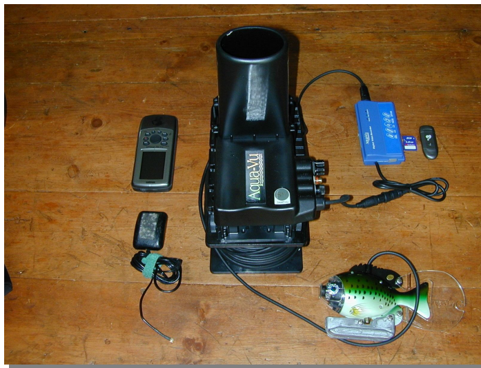
Underwater camera equipment used to observe Lake Geraldine.
