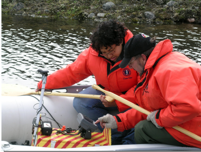
Christian Prévost teaches LeeAnn Pugh of the Nunavut Department of Environment bathymetric survey techniques.
