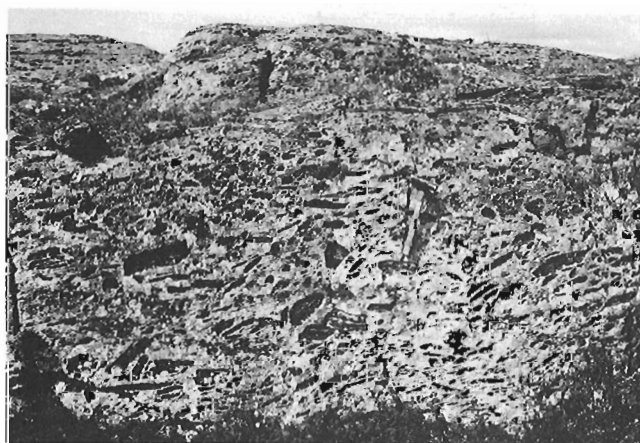
Figure 5. Intraclastic breccia unit 1.8 m thick containing clasts selectively replaced by carbonate (dark). Matrix is poorly sorted coarse volcarenite. GSC 205025-G.
