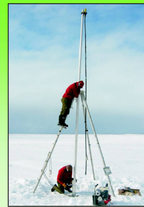
Photos: drilling through sea ice, setting up vibracore, and lab work
