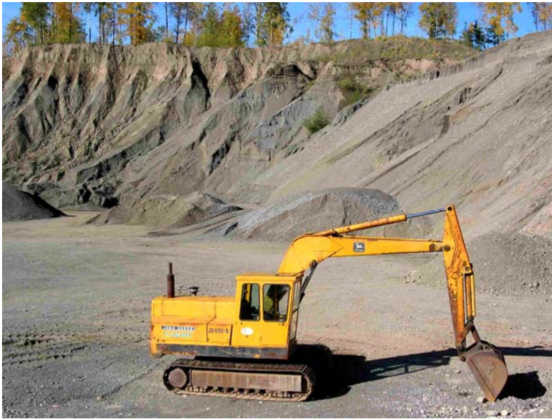
Figure 24. A gravel pit in an Ice Age bench along Highway 16 just east of the Kitsumkalum River bridge. The cliff exposes thick sand and gravel deposits (grey) overlain by a 3-5m layer of clay and silt (tan). Photo by Bob Turner.
