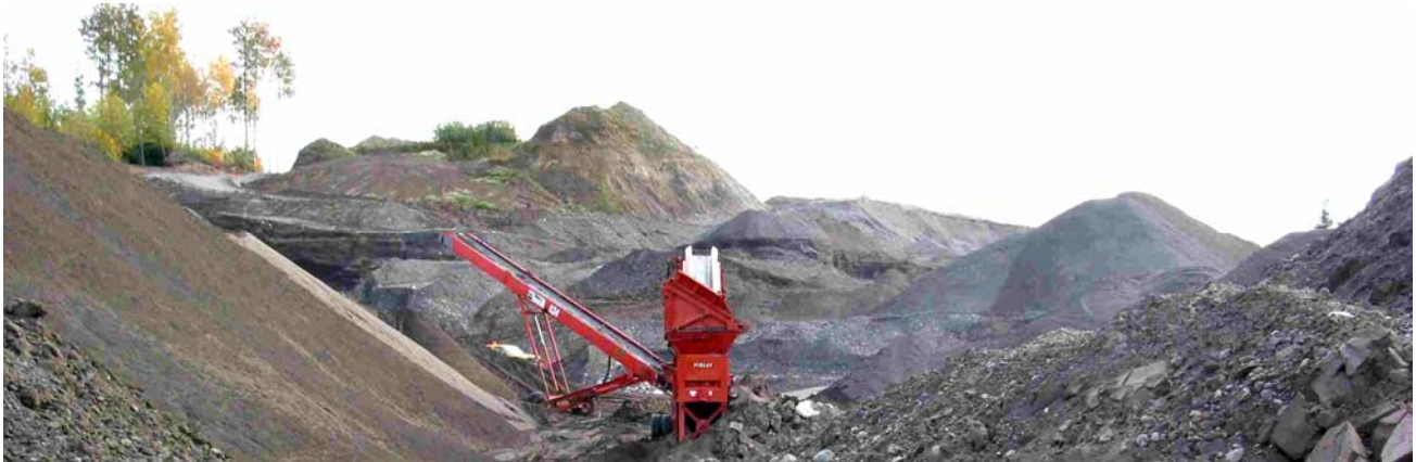
Figure 25. (below) A gravel pit along Highway 16 near the Kitsumkalum River. Sand and gravel deposits are sorted by screening into separate piles of gravel and sand, and each is sold for different purposes. Photo by Bob Turner.
