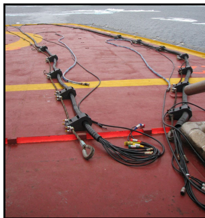
Figure 5.4 Two assembled tow bundles showing pull cables, bundles, with clamps fitted.
