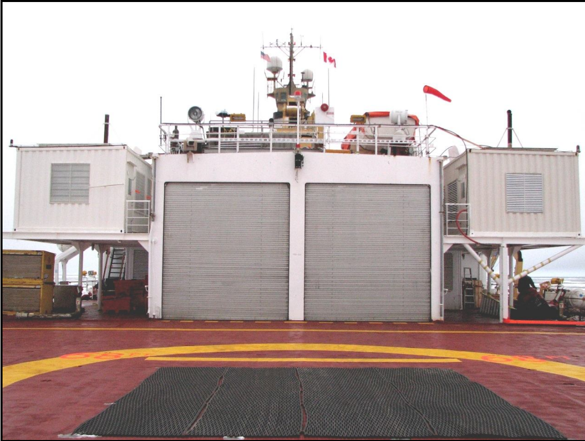
Figure 5.12 From flight deck showing both compressor containers as fitted in 2008.
