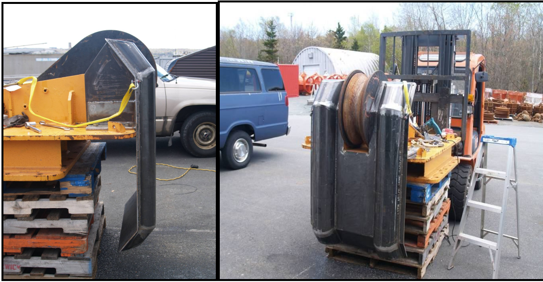
Figure 5.7 Early 2008 picture taken at the fabrication yard showing the newly fitted fairlead system attached to the LSSL aft roller sheave and base.
