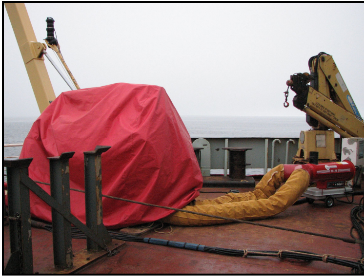
Figure 5.16 Herman Nelson-type heater supplying a steady flow of warm air to the port sled system.
