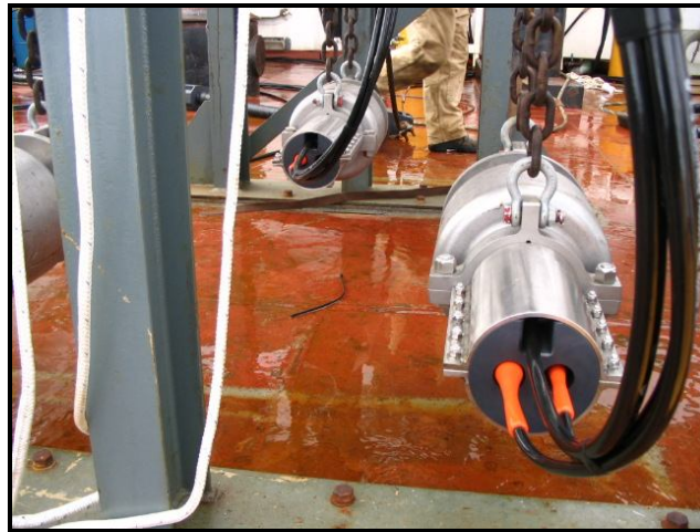
Figure 5.10 10 520 cubic inch gun with collar protectors fitted.
