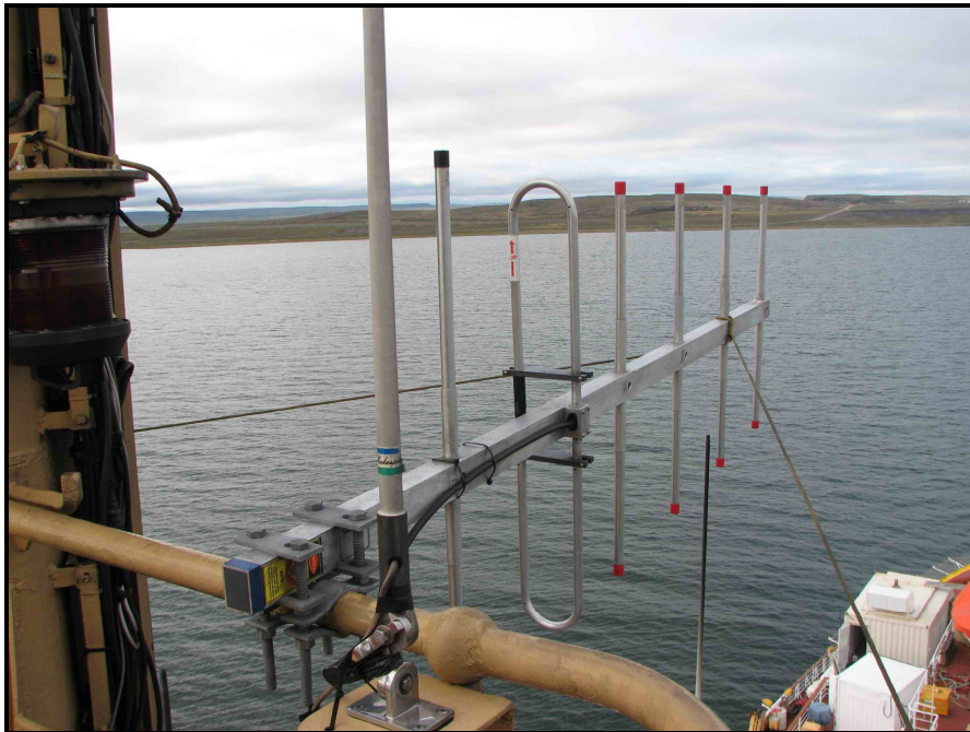
Figure 5.22 Sonobuoy antenna as fitted in 2008.
