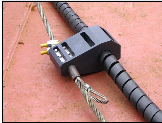
Figure 5.3 Pull cable showing one of the eyelets used for deployment and recovery.
