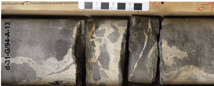
Core 6: Anhydrite-filled fractures
