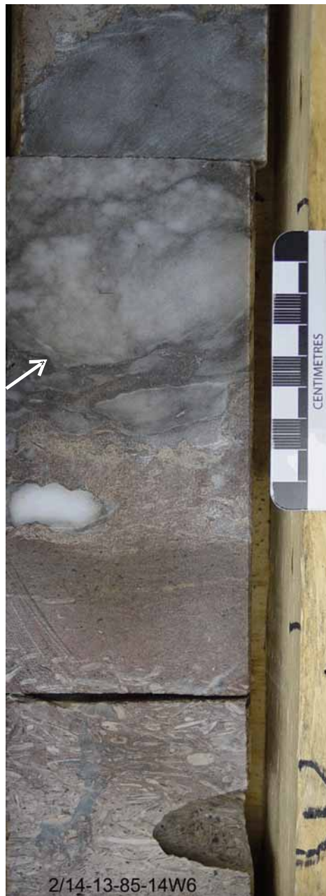
2/14-13-85-14W6 Charlie Lake Fm: interval 1386.45 - 1387.5 m. and contact with overlying anhydrite bed
