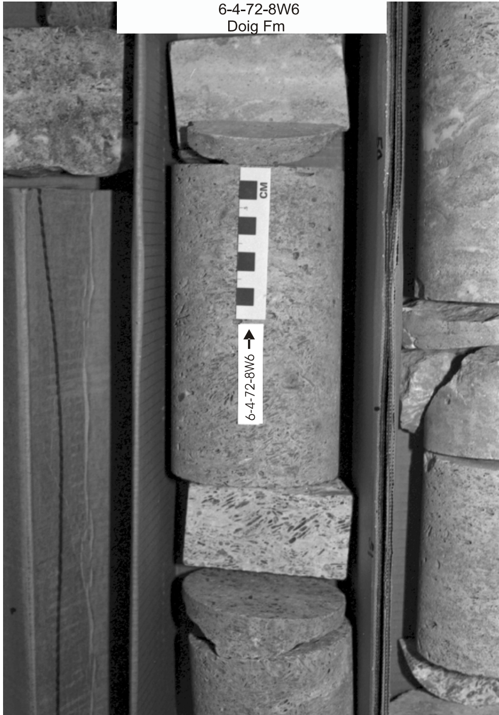
Coquinal sandstone in the Doig Fm at about 2317 m
