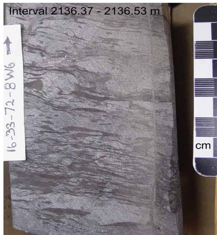
Irregular clay laminae and clay lenses in an ATSB in the Doig Fm
