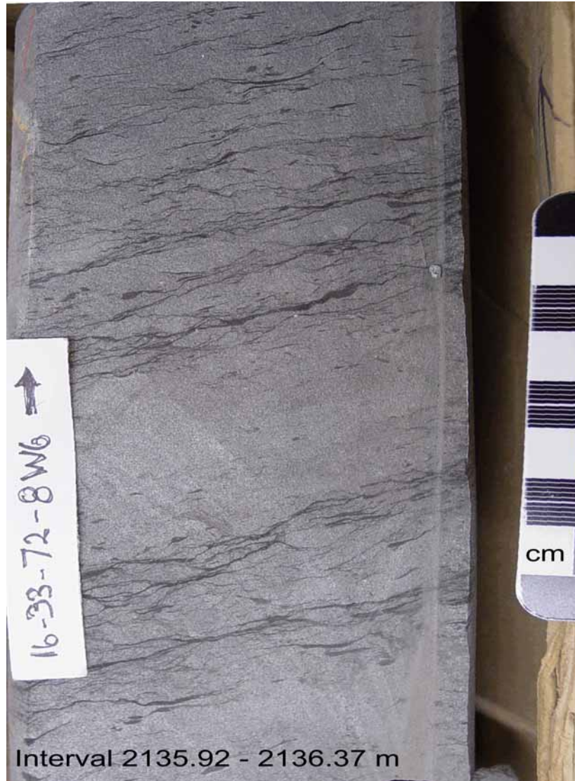
Irregular clay laminae in an ATSB in the Doig Fm
