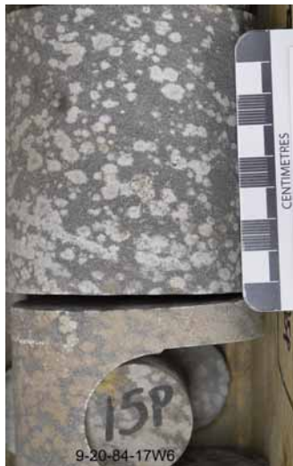
Interval 1253.47 - 1256.73 m Unstained Cecil Mbr with incipient anhydrite cement
