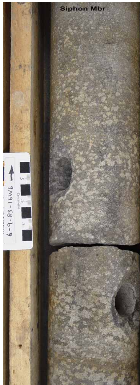
Mottled sandstone of the Siphon Mbr (probably due to anhydrite/dolomite cementation). Interval 4207' 2" - 4208' 4"
