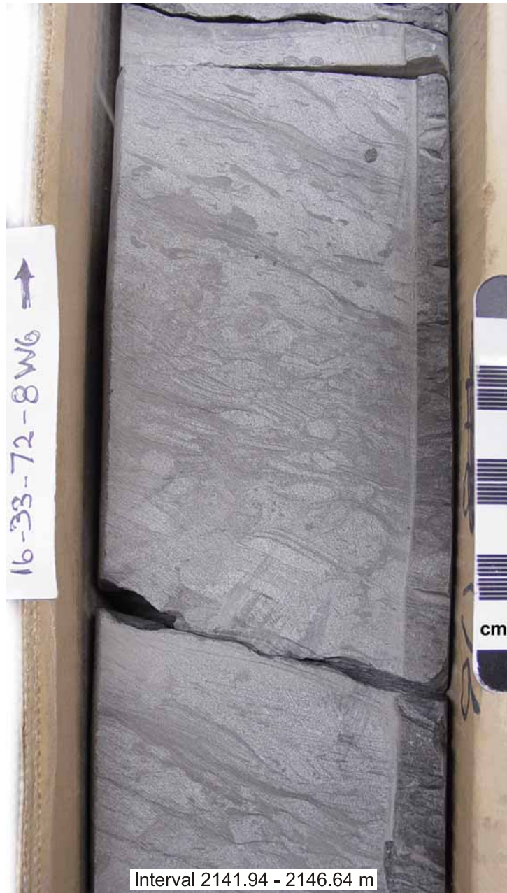
Burrows and over-steepened beds in an ATSB in the Doig Fm
