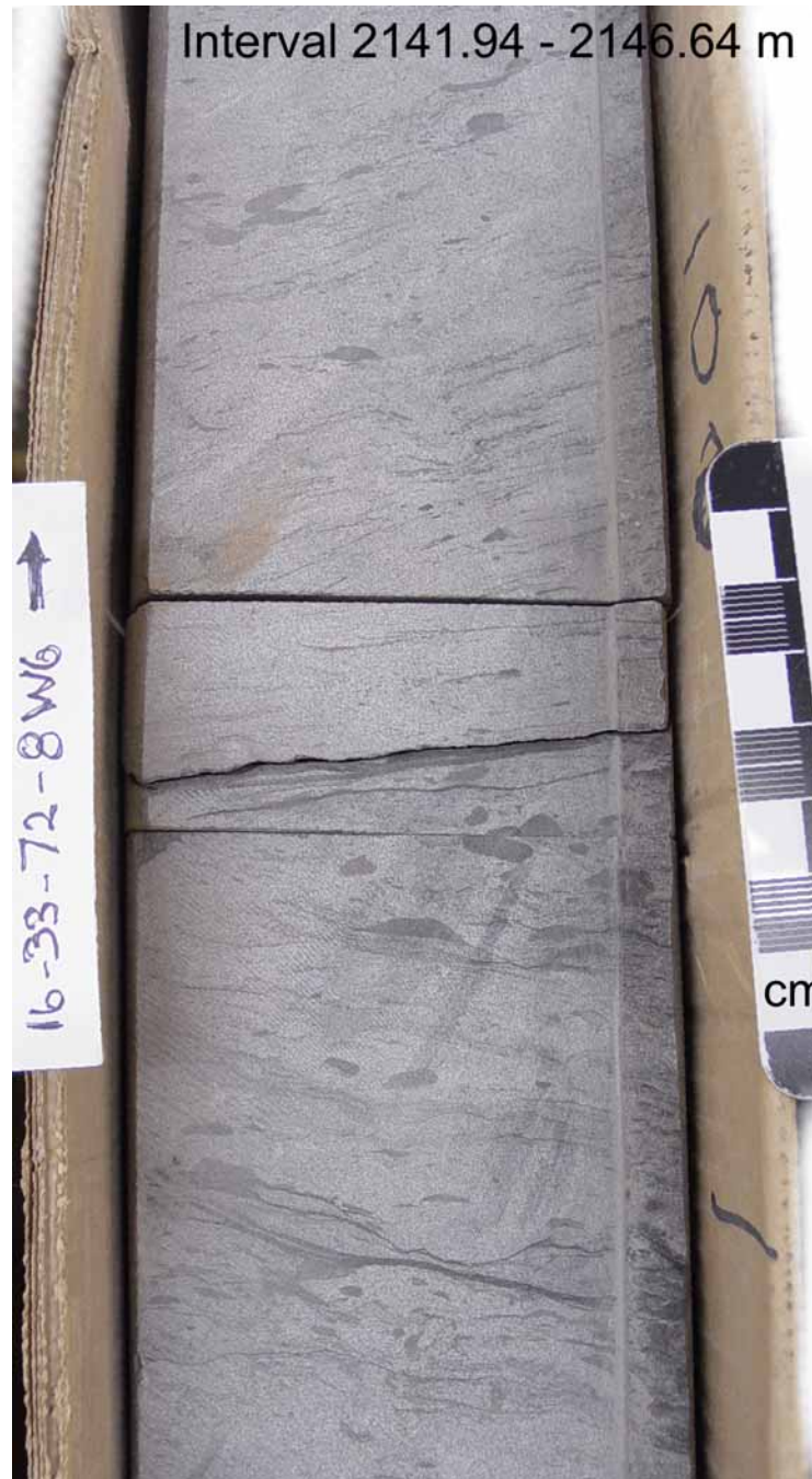
Irregular clay laminae and clay lenses or clasts in an ATSB in the Doig Fm
