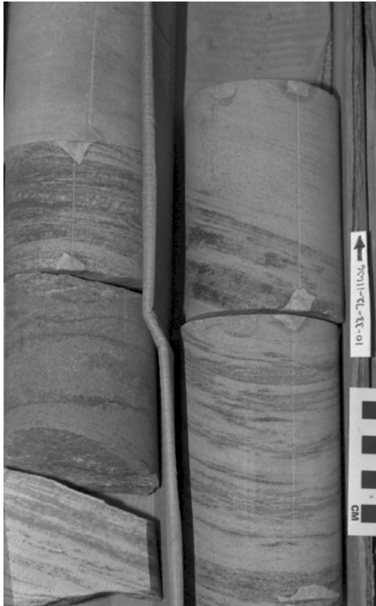
Halfway Fm.: cross beds highlighted by incipient anhydrite/dolomite cement. (interval 2491.51 - 2496.1 m)
