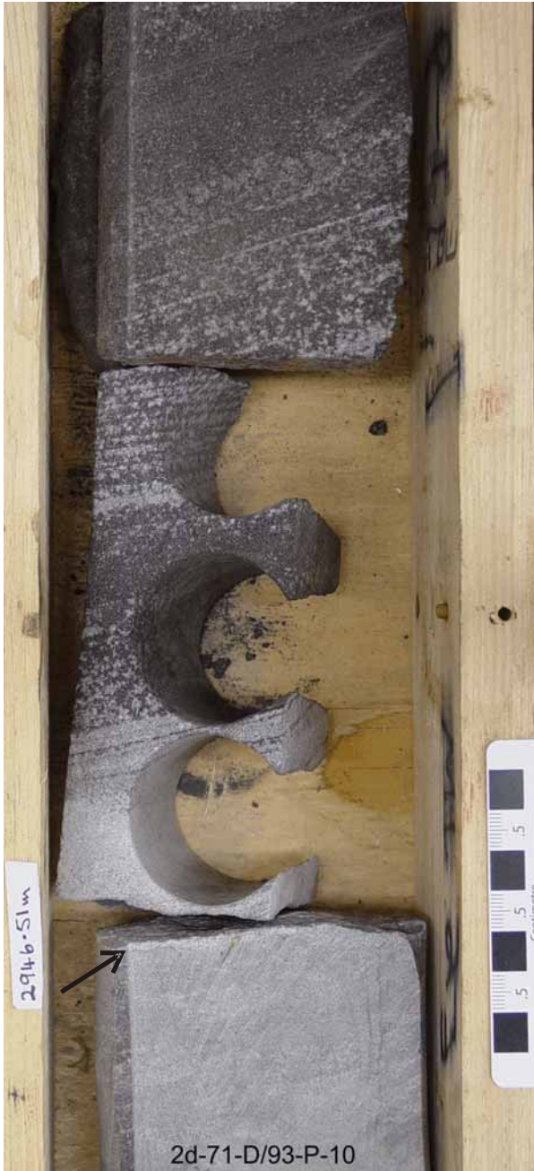
Oil stained Artex Mbr above basal contact at 2946.51 m
