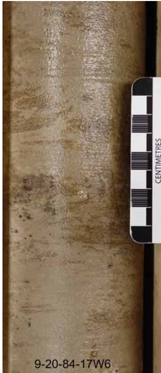
Interval 1253.47 - 1256.73 m Oil stained Cecil Mbr. Core piece from near top of member
