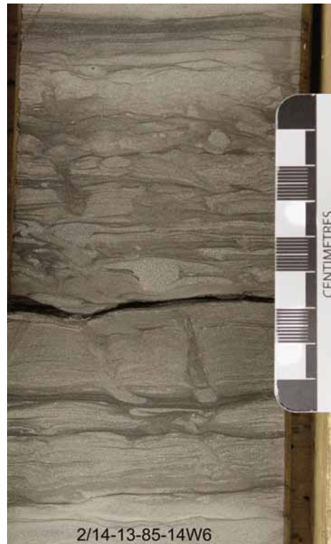
?Halfway Fm: interval 1396.73 - 1398.2 m. Burrowed, laminated sandstone.
