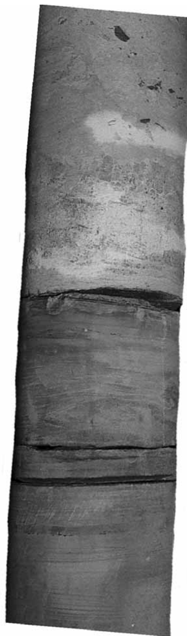
Load deformed dolomitic mudstone, Charlie Lake Fm (interval 1468.97 - 1469.65 m)
