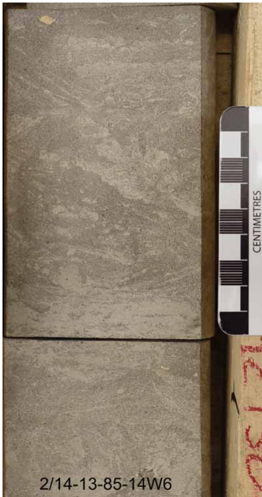
Halfway Fm: interval 1389.44 - 1390.88 m. Dolomite mottled sandstone
