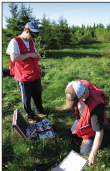
Step 13. Attaching the soil gas filled syringe to the evacuated IC and recording the time the IC was filled on the data sheet.
