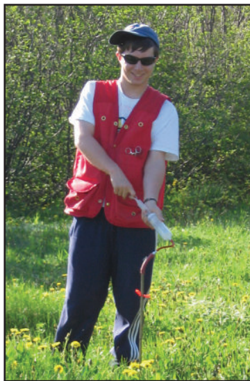
Steps 9 and 11. Extracting soil gas with the syringe attached to the small tube.
