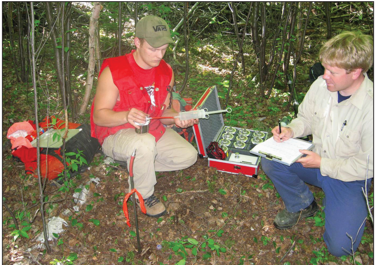
Figure 4-3. Top - Collection of soil gas sample from hollow steel probe using a 150 ml syringe. Probe was inserted 60 cm into the soil. Bottom - Gas sample in syringe is transferred from the syringe into the ionization chamber. (Photos by K. Ford)
