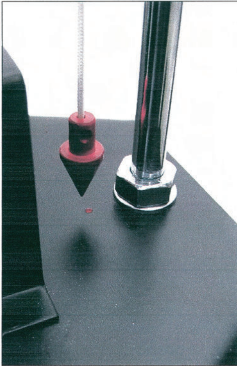
Fig. 17: The plummet used for leveling the equipment in situ, basic plate horizontal
