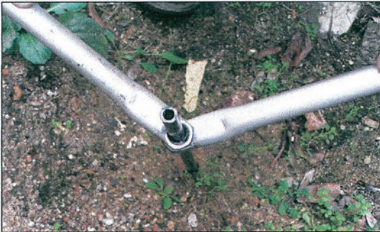
Fig. 20: Set up for retracting – simple retractors
