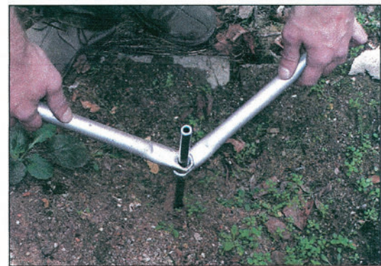
Fig. 21: Retracting the probe to the surface using simple retractors
