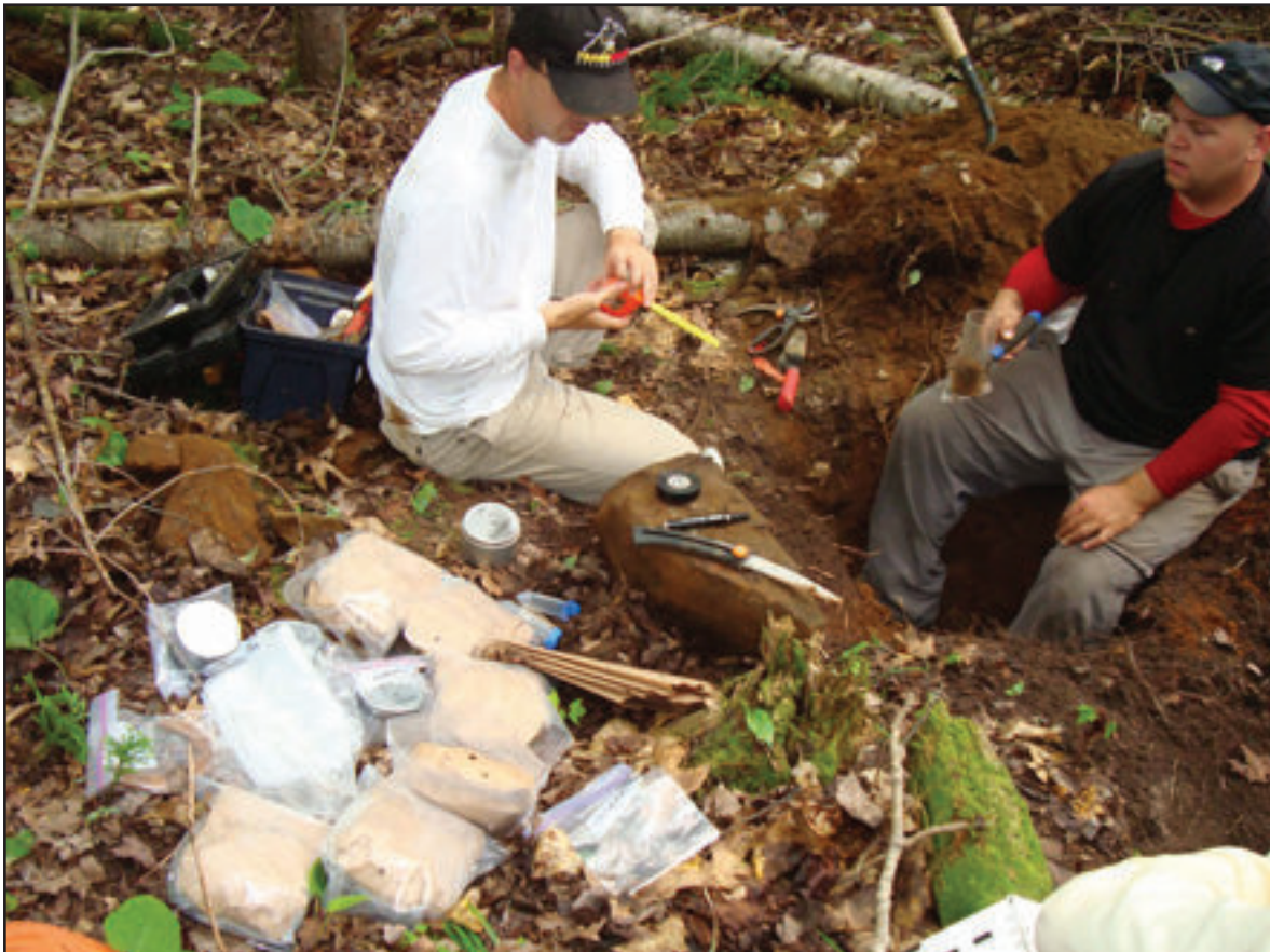
Collecting soil samples from the “public health” layer and A-, B- and C-horizons near Pembroke, Ontario, in summer 2008. (Photo by I. Kettles)
