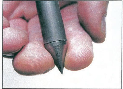
Fig. 2: Inserting the sharp tip into the lower end of the sampling probe (2)
