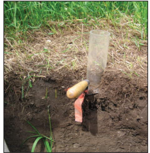
Step 2 - Press the sampler into the soil.
