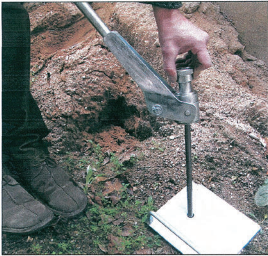
Fig. 25: Set up for retracting – the special retractor for easy retracting to the surface
