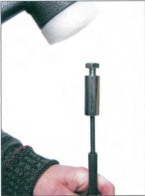
Fig. 9: The sharp tip is moved to the exact distance using the punch wire and the adjusted distance screw
