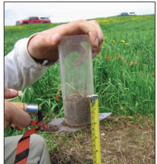
Step 3 - Remove the sampler using the trowel, if necessary.
