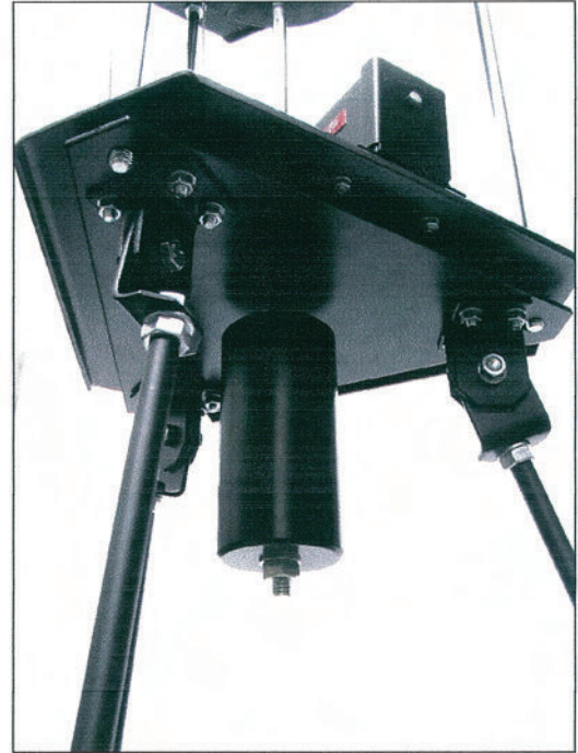
Fig. 18: Attachment of the first weight to the tie rod of the equipment, the initial state of sack in the upper constricted position
