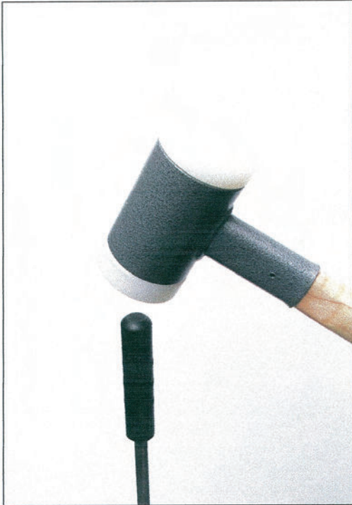
Fig. 5: The probe is pounded to the desired depth using the special hammer and the drive in head
