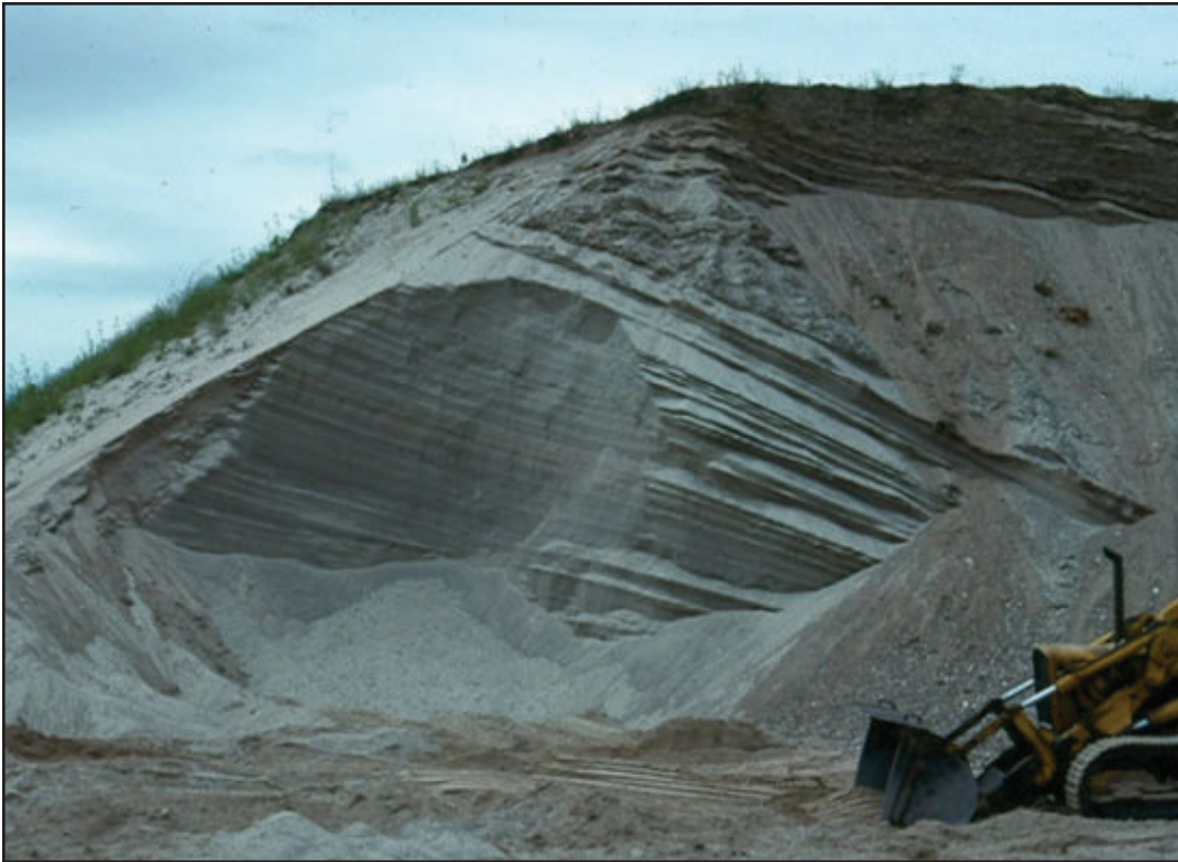
Figure 5-5. Borrow pit in Eastern Ontario where glaciofluvial sand and gravel are being excavated.
