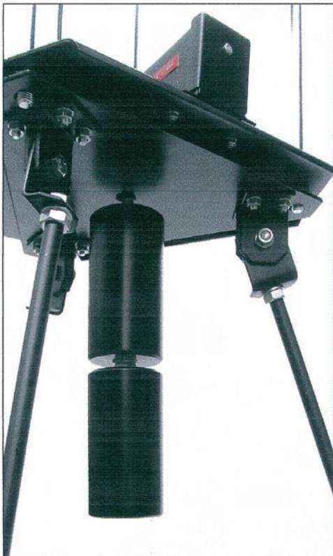
Fig. 19: Screwing the second weight
