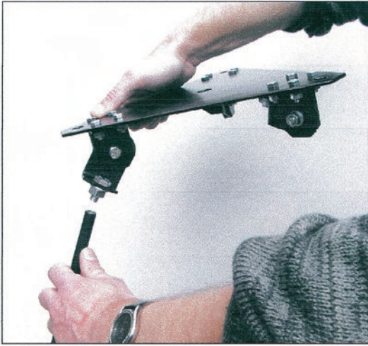
Fig. 13: Making the tripod mount
