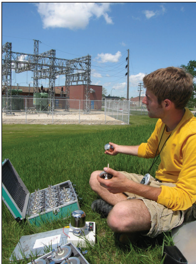
Measuring soil gas radon in Manitoba (Photo by. H. Byker)
