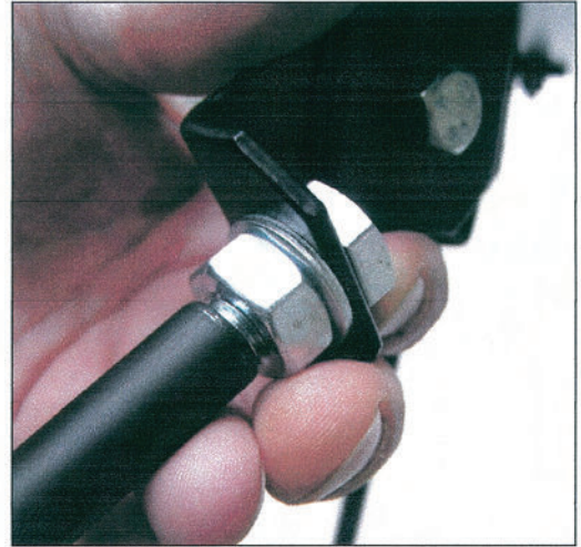
Fig. 14: Screwing the tripod leg
