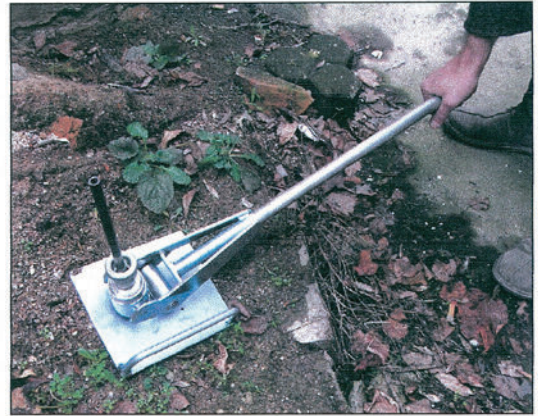
Fig. 26: Retracting the probe to the surface using the special retractor
