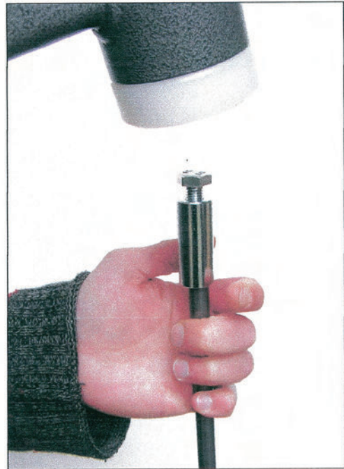
Fig. 10: The sharp tip is moved to the exact distance – the defined measurement surface is opened
