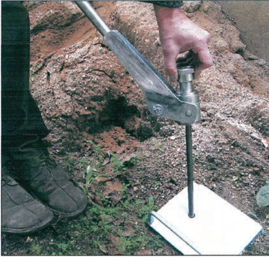
Fig. 18: Set up for retracting – the special retractor for easy retracting to the surface
