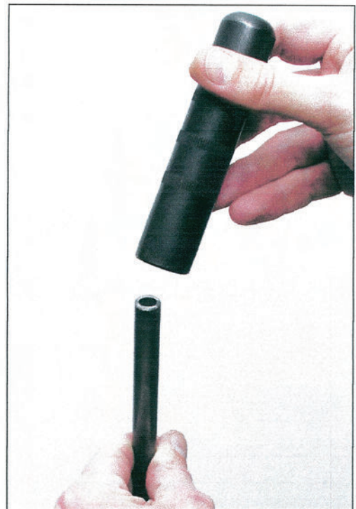
Fig. 4: Preparing the drive in head
