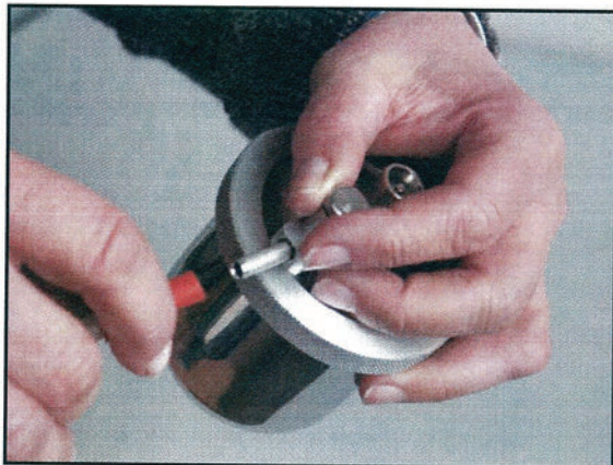
The photo sequence (the transfer of the soil gas sample into the ionization chamber)
