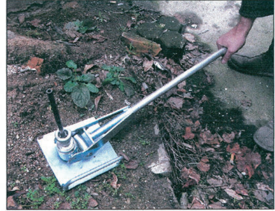
Fig. 19: Retracting the probe to the surface using the special retractor
