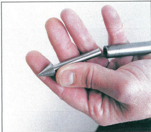
Fig. 1: Inserting the sharp tip (special type for permeability measurements) into the lower end of the sampling probe (1)
