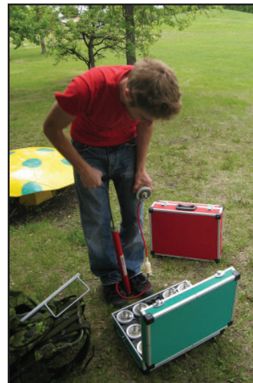
Step 1. Pumping out the ICs with the modified pump.
