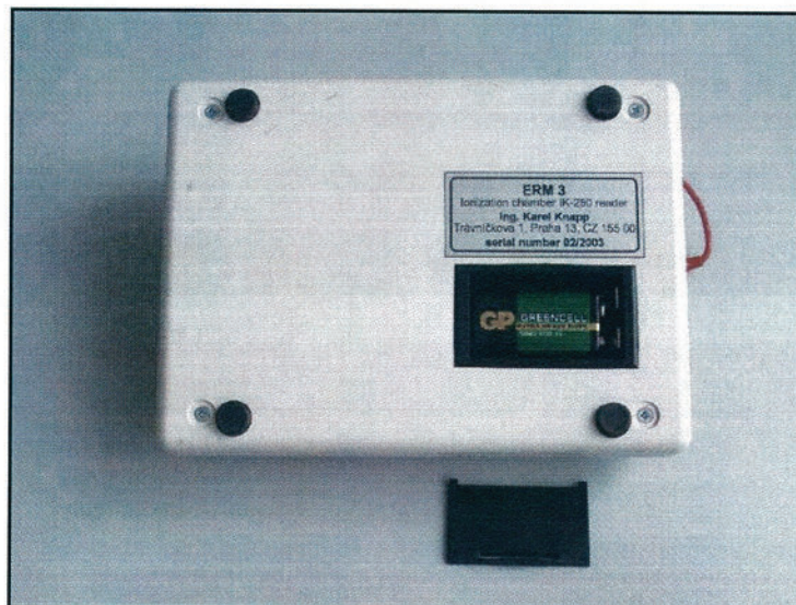
Picture E. The battery slot of the electrometer
