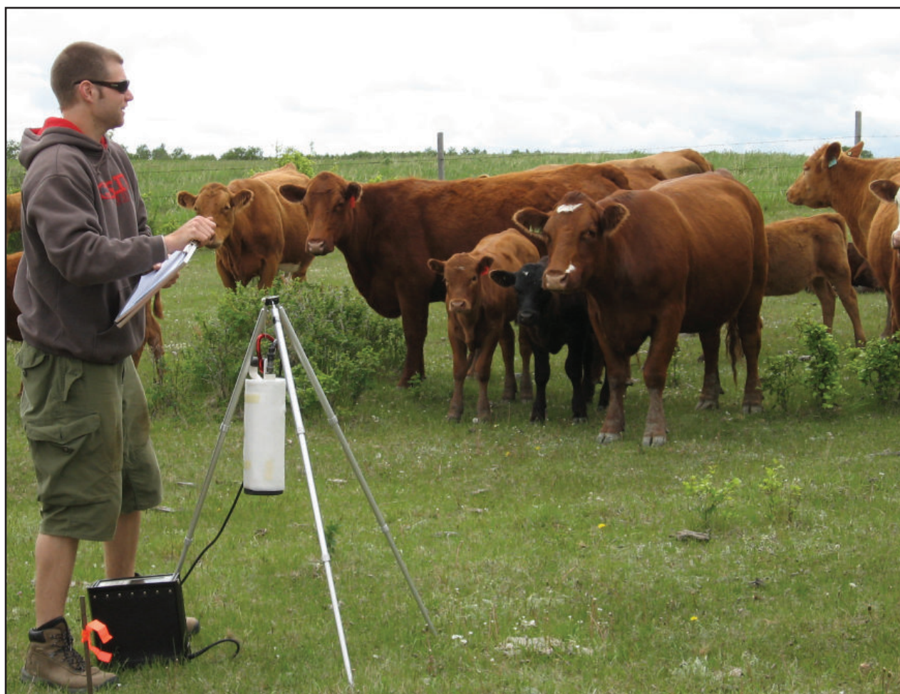
Measuring soil gas radon and natural radioactivity in southern Saskatchewan. (Photo by J. Campbell)
