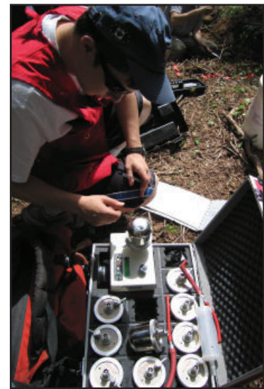
Step 16. Taking a reading of the radon concentration collected from the soil gas.
