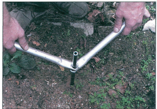
Fig. 28: Retracting the probe to the surface using simple retractors
