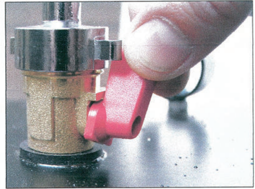
Fig. 22: The suction is started by opening the cock to the full, the time interval between two acoustic and/or light signals is measured
