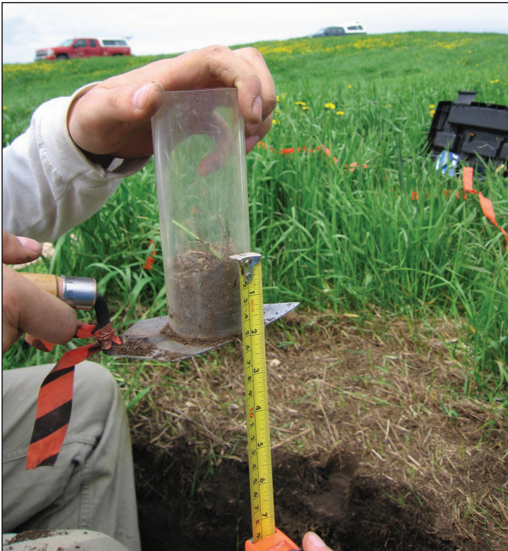
Bulk density sample collected from the “public health” layer (0-5 cm) in Gaspé, Québec. (Photo by R. McNeil)
