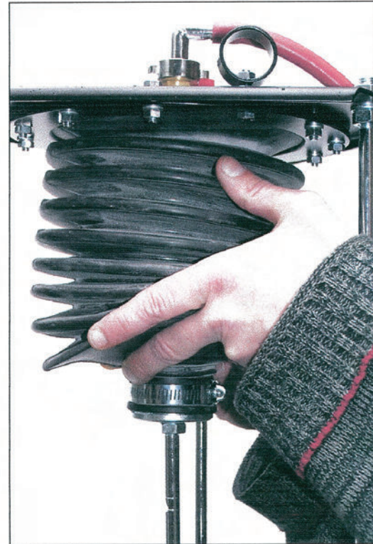
Fig. 24: The sack is returned to the upper contracted position, then the cock is again closed
