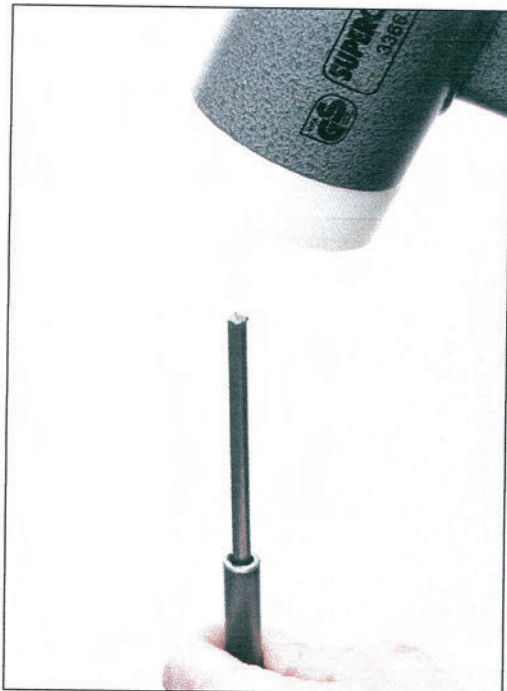
Fig. 7: The sharp tip is moved a few centimetres lower, which makes a cavity at the lower end of the probe
