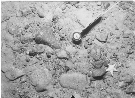
Figure 2b - gravel facies of the Sable Island Sand and Gravel unit.
