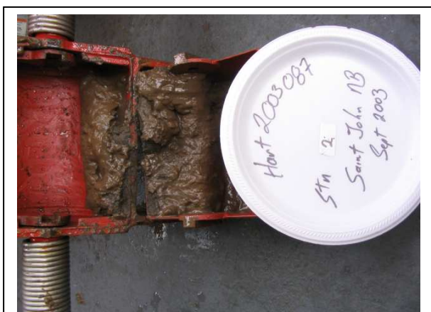
Figure 3. Seafloor samples were collected during survey Hart 2003097 with a Shipeck grab sampler, shown here.
