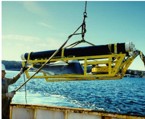
Figure 4. Seistec sub-bottom profiler showing the surface-towed catamaran used to support the boomer and line-and-cone array. Power and signals are contained in the tow cable bundle on the front of the catamaran.
