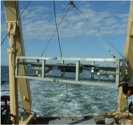
Figure 7. Icehole camera used to collect seafloor photographs during Hart 2003015.
