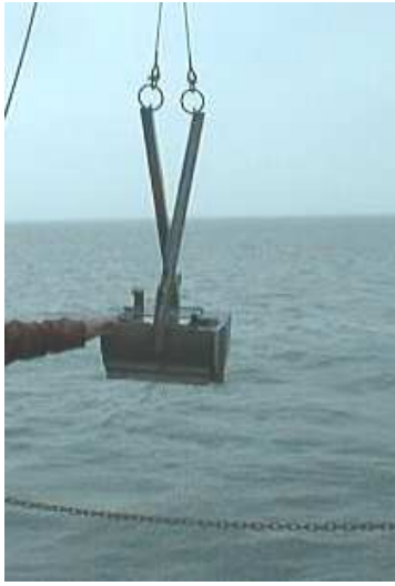
Figure 5. Seafloor samples were collected during with a van Veen grab sampler.
