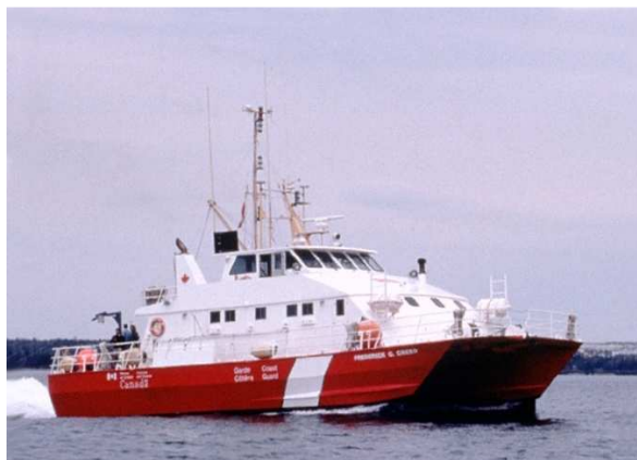
Figure 1. Multibeam bathymetry, sub-bottom profiler and magnetic data were collected using the CCGS Frederick G. Creed equipped with a Kongsberg EM1002 multibeam bathymetry system.
