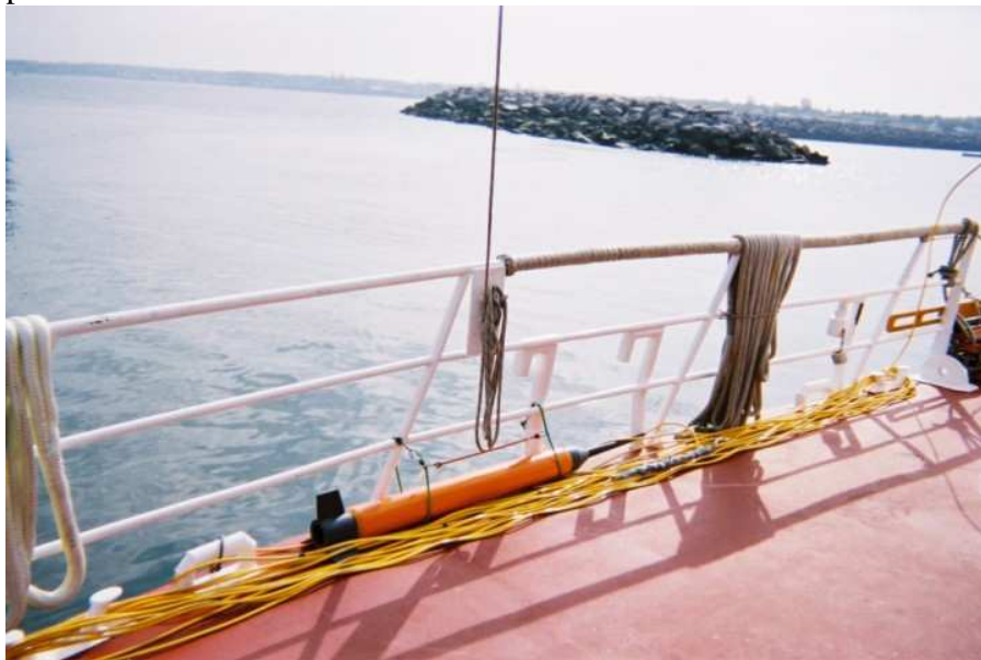
Figure 2- Setup of magnetometer while on deck.
