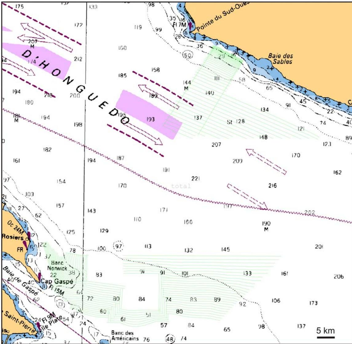
Figure 3: Survey lines for the 2009 Honguedo Survey. Line spacing was dependant upon water depth, target feature resolution and tide. Survey line spacing ranges from approximately 1000m in deep water, to approximately 100m in the shallowest section (Site A).
