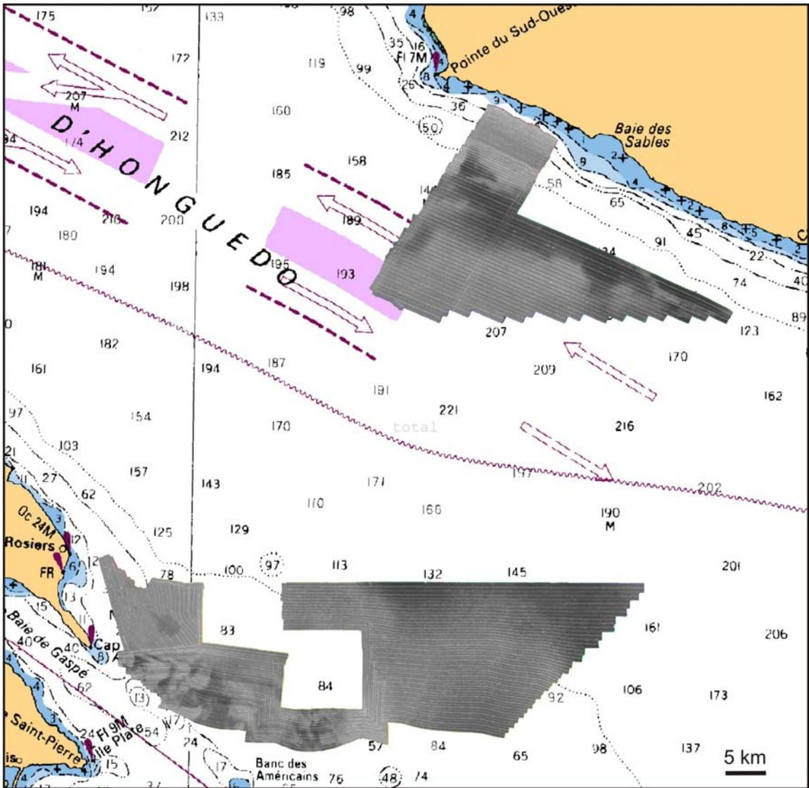
Figure 5: Backscatter data extracted from multibeam bathymetry data.
