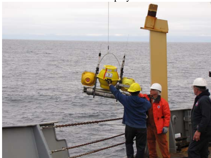
Figure 8. OBS during recovery (photo courtesy of GSC).
