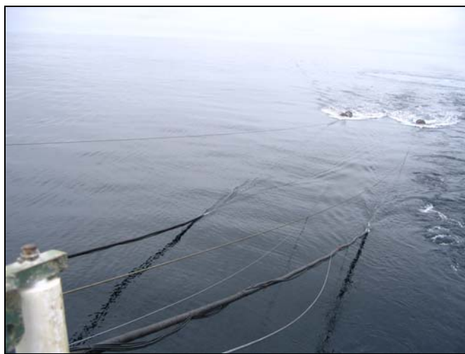
Figure 18. Starboard air-bundle cables, electrical lines and recovery wires.
