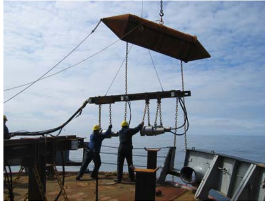
Figure 46. Deployment of airgun array. Photo: Thomas Funck.
