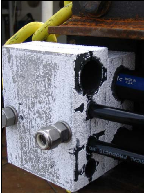
Figure 16. Shown here are two of the nine breakout or pass-through blocks located on each array beam. Those shown are located on the forward port side of the beam.
