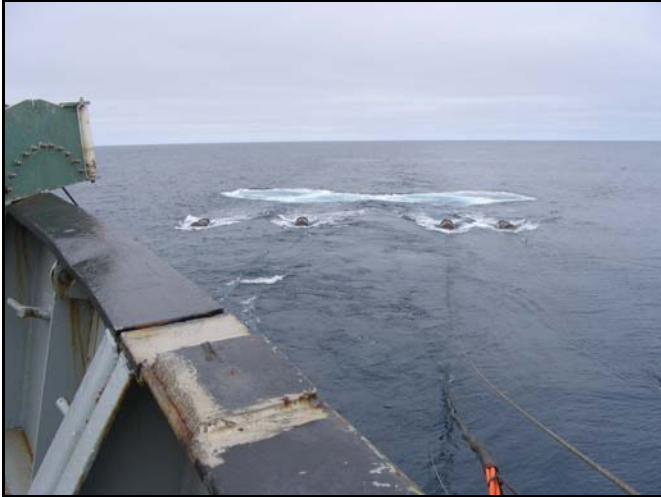
Figure 19. Image showing the four surface floats towed from Hudson's quarterdeck area.
