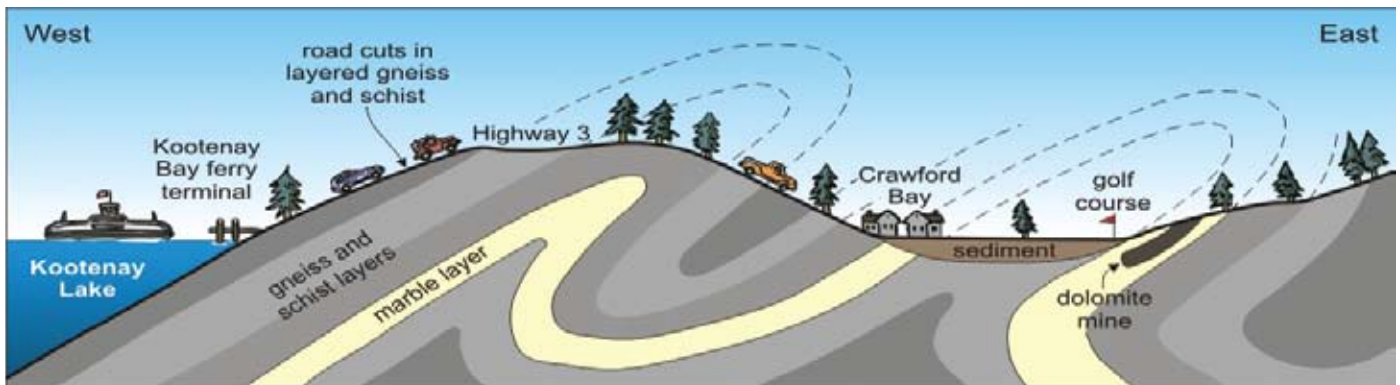
Figure 27. A schematic cross section of Highway 3A from Kootenay Bay to Crawford Bay showing the large scale folds of rock layers due to tectonic collision 170 million years ago.
