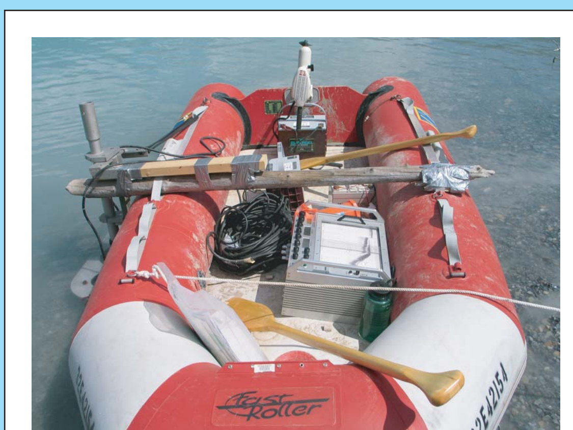
Fig. 3. The Zodiac Fastroller 310, with the Knudsen 320M™ sub-bottom profiler and 12V batteries, loaded and ready to go.
