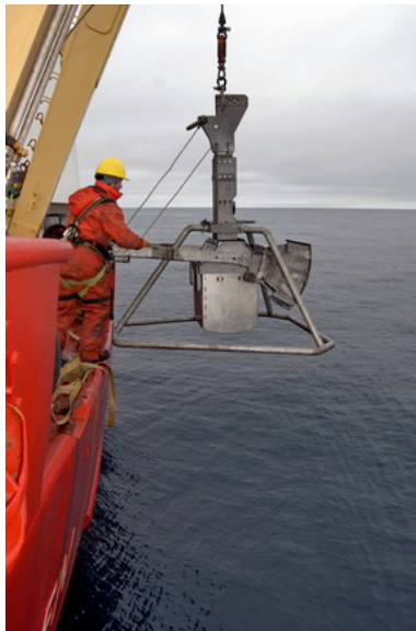
Figure 3 – Photo of box corer used onboard the Amundsen in 2006 (photo courtesy Keith Lévesque, ArcticNet)
