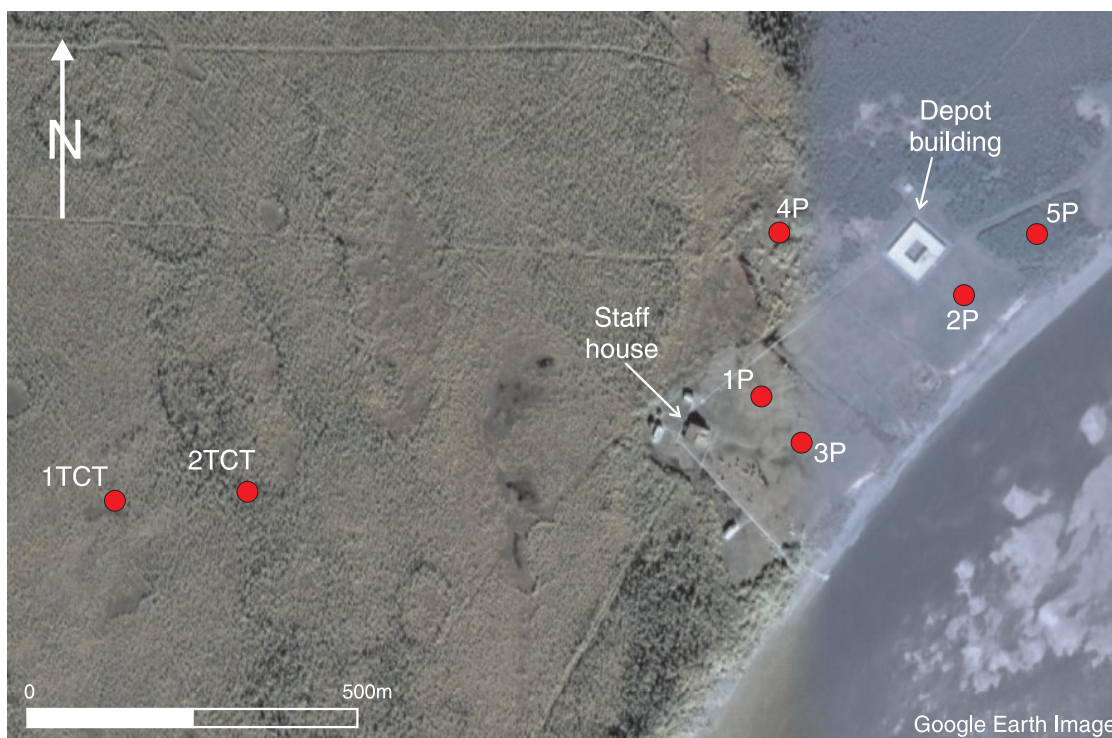
Figure 2. Location of boreholes and temperature cables.
