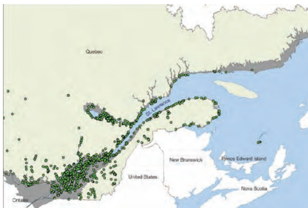
FIGURE 22: Inventory of requests to respond to landslides in Quebec between 1972 and 2005. The grey zone shows the limits of the postglacial marine transgression that left clay deposits (map provided by the Ministère des Transports du Québec, pers. comm., 2006).
