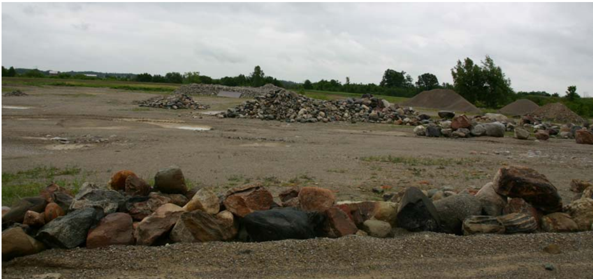
Figure 42. Illustrative photograph of largely worked out and partially rehabilitated shallow (< 3 m deep) Spivak pit with isolated piles of oversized unprocessed boulders and cobbles
