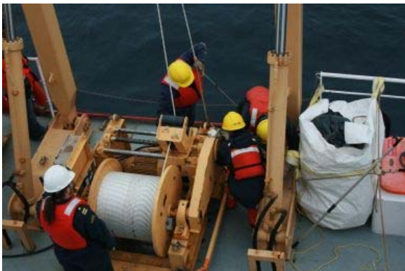
Figure 4: a) tying off rope to allow slack for free-fall b) Throwing slack and cutting tether for freefall
