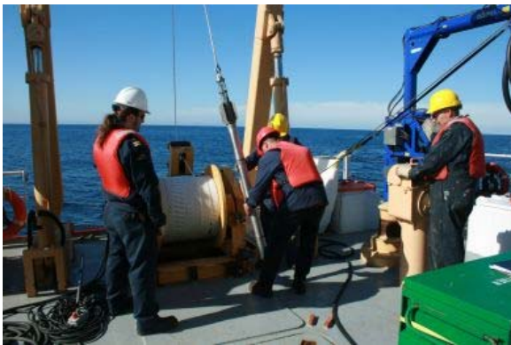
Figure 3: a) FFCPT probe and winch with 350 m rope b) Deploying FFCPT through A-frame
