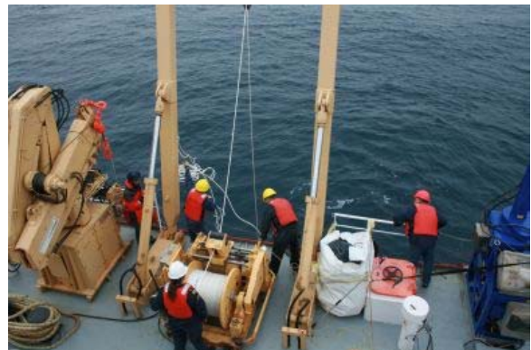
Figure 4: a) tying off rope to allow slack for free-fall b) Throwing slack and cutting tether for freefall
