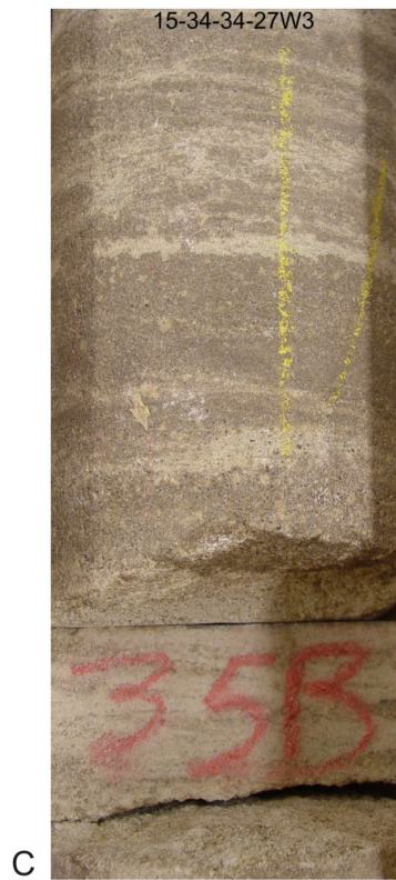
Cross bedded medium to granular sandstone
