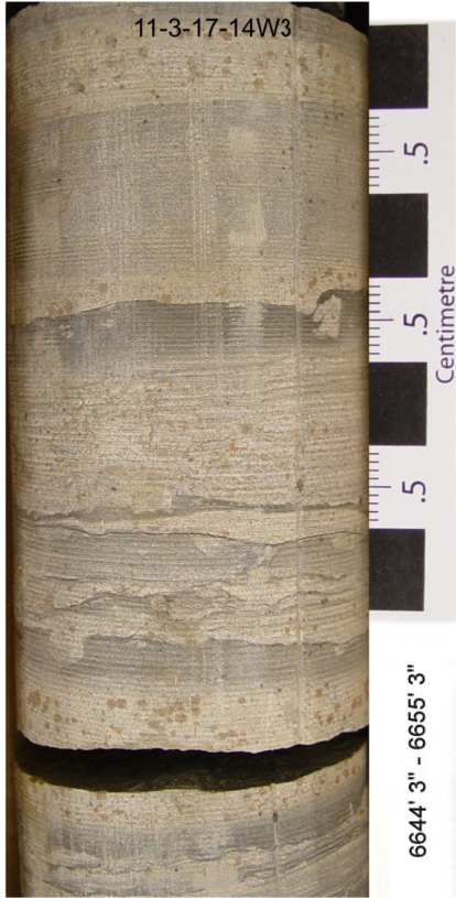
A. Interbedded burrowed sandstone and mudstone
