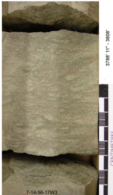
D. Burrow mottled, glauconitic, argillaceous sandstone
