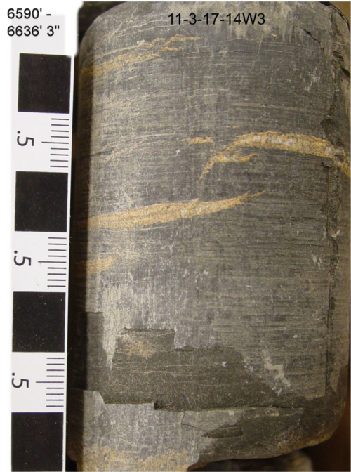
A. Horizontal fractures in shale
