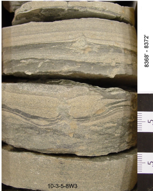
A. Thin interbeds of laminated sandstone and burrowed mudstone.
