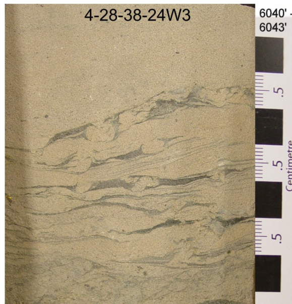
B. Burrowed sandstone and mudstone
