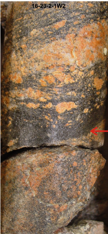
C. Contact with basement granite at 2800.78 m
