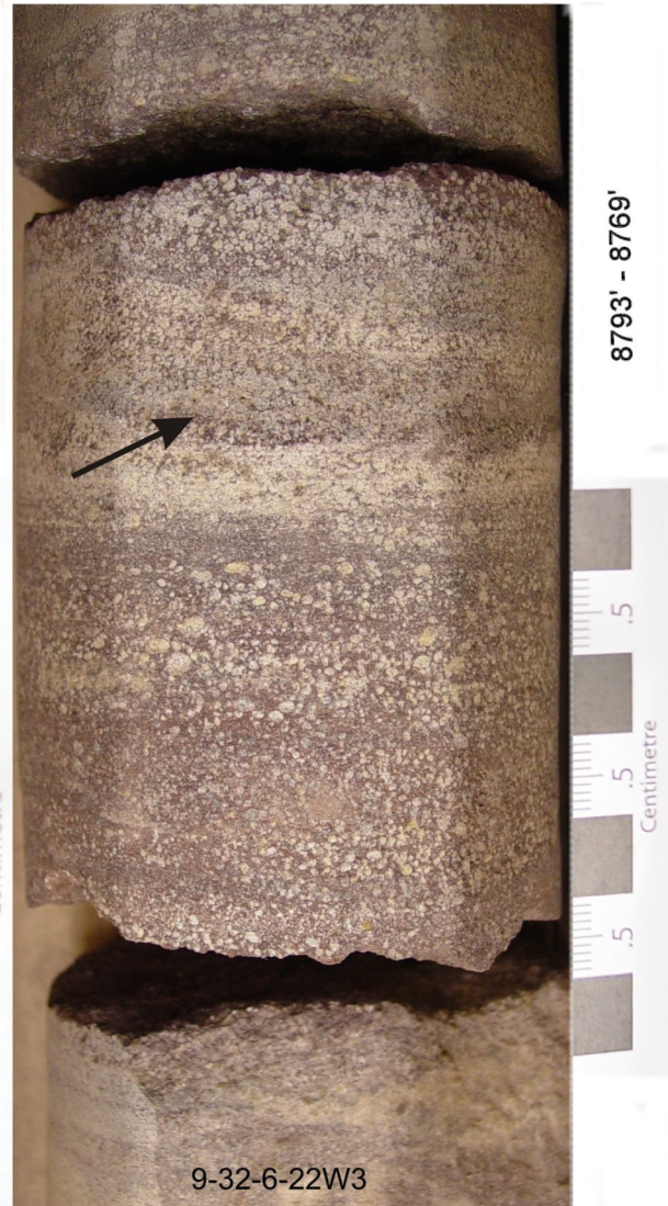
B. Large-ripple cross-laminae (arrow) in arkosic sandstone
