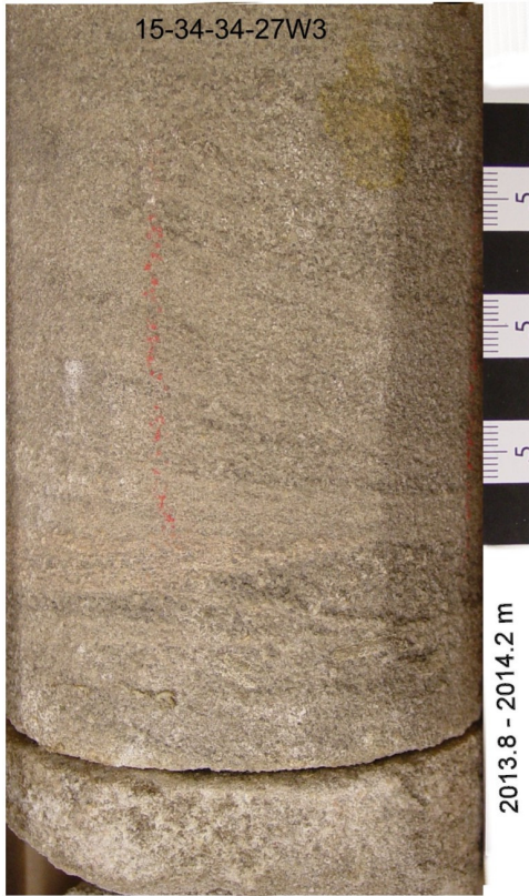
A. Cross bedded, coarse-grained sandstone
