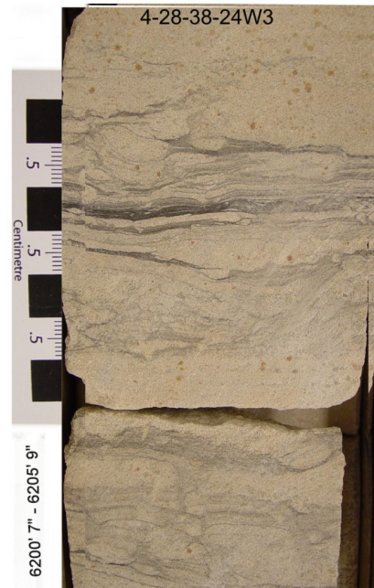
D. Burrowed, interbedded sandstone and mudstone
