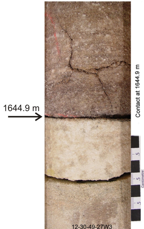
D. Contact between a red and a white sandstone interval
