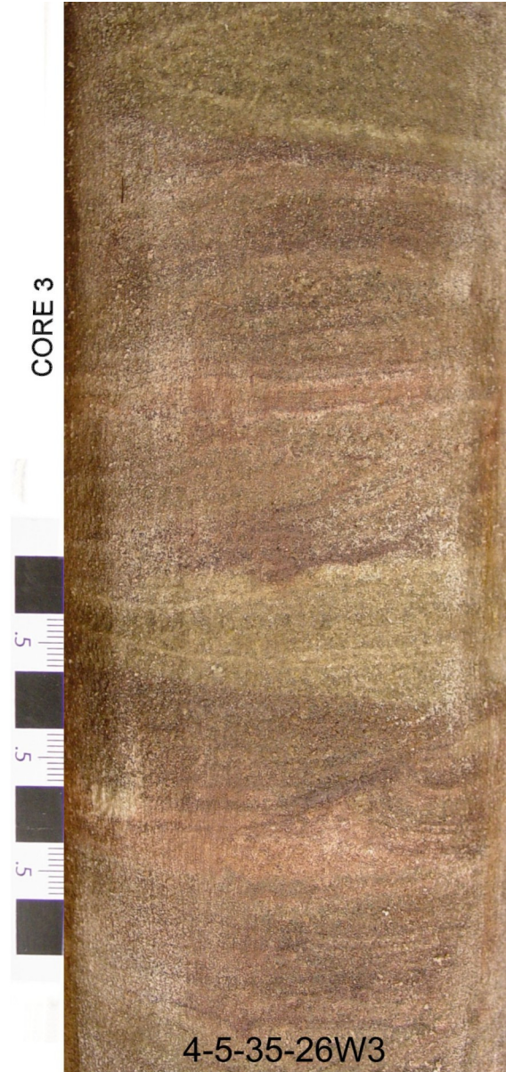
B. Cross beds and ripple laminae in red sandstone
