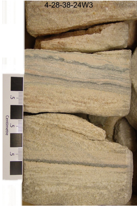
B. Core 18: thin mudstone layers separating sandstone beds
