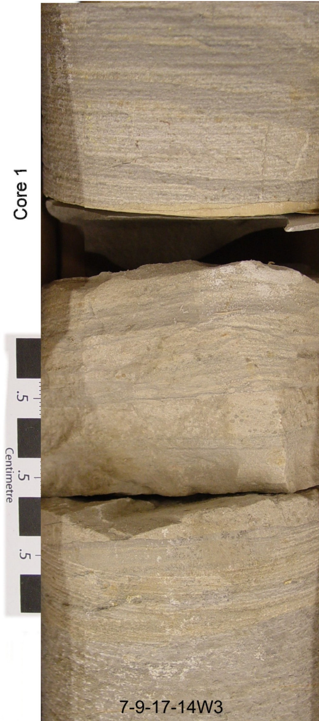
Very thin interbeds of siltstone and silty sandstone
