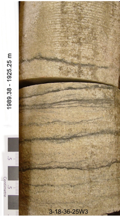
D. Thin sandstone beds separated by mudstone laminae
