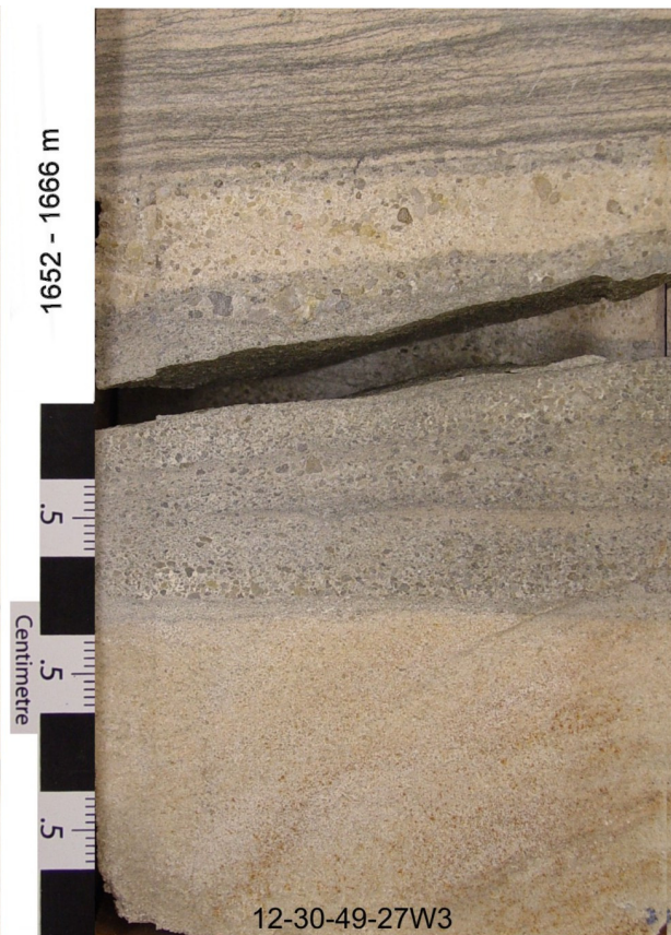
B. Thin beds of coarse-grained to granular sandstone
