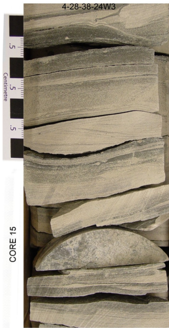
D. Ripple laminated sandstone interbedded with mudstone
