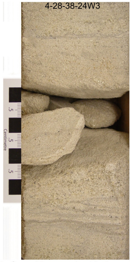
D. Core 18: cross bedded sandstone
