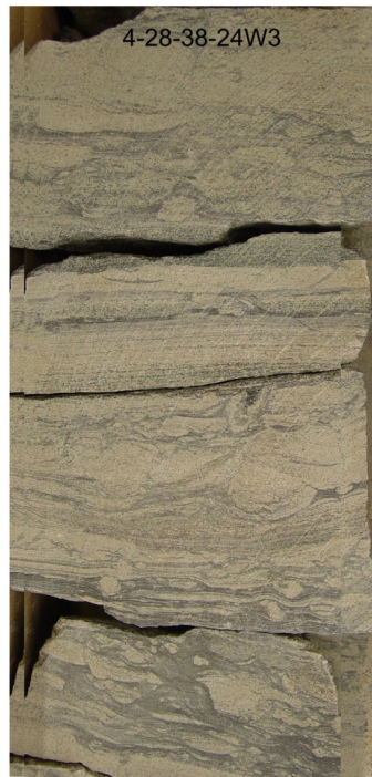
E. Interbedded burrowed sandstone and mudstone
