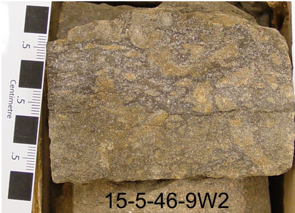
2527' 7" - 2528' 7": burrowed sandstone immediately overlying granite basement
