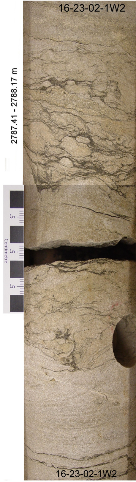
B. Interbedded burrowed and cross bedded sandstone
