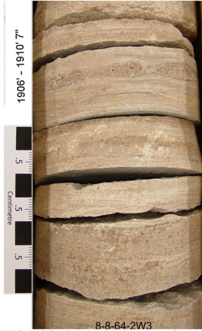
A. Interbedded sandstone and mudstone with scattered beds of coarse-grained sandstone
