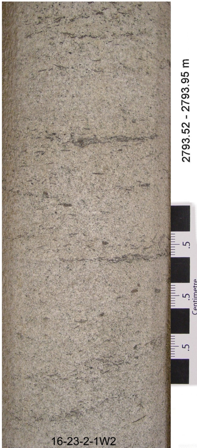
A. Cross bedded sandstone with mud clasts
