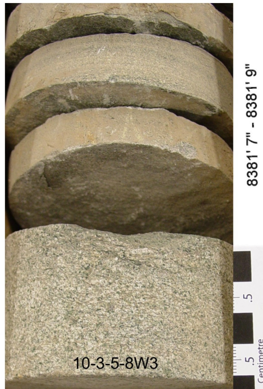
D. Isolated bed of coarse-grained sandstone
