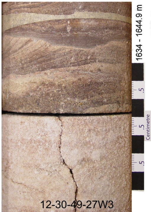
C. Ripple laminated sandstone overlying cross bedded sandstone
