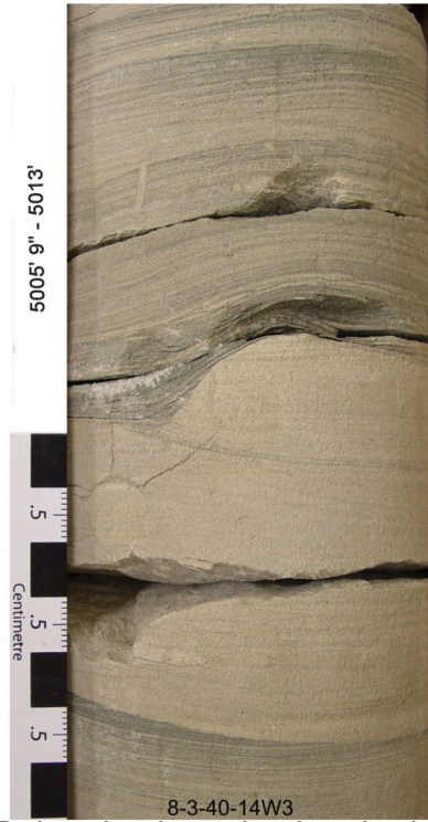
B. Interlaminated to interbedded mudstone and sandstone
