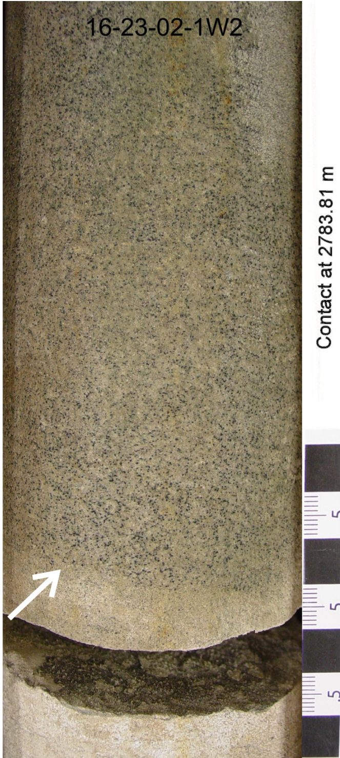
A. Basal bed contact (arrow) at 2783.1 m
