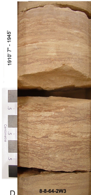
Very thin interbeds of sandstone and mudstone with some burrow structures.
