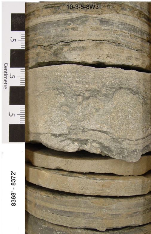
C. Thin interbeds of sandstone-mudstone with thicker bioturbated bed.
