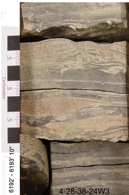
C. Interbedded, burrowed, mudstone and sandstone
