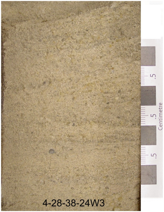
C. Core 18: cross bedded sandstone
