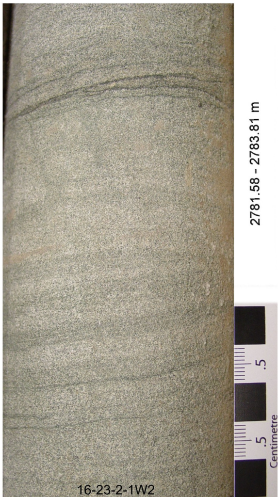
C. Cross bedded sandstone with mud laminae
