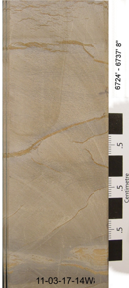
B. Well cemented siltstone to very fine grained sandstone
