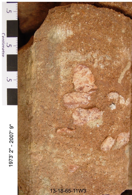
C. Small angular pebbles of feldspar in arkosic sandstone
