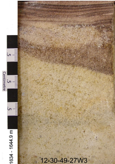
B. Clay laminated sandstone overlying cross bedded sandstone
