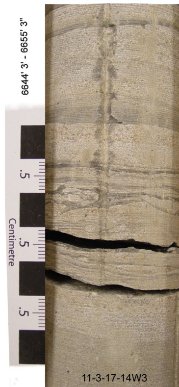
D. Scattered burrowed beds in sandstone
