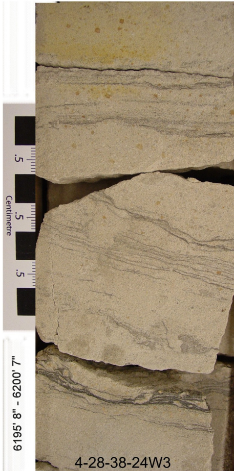
A. Thin sandstone beds separated by mm-thick mudstone layers. Minor bioturbation
