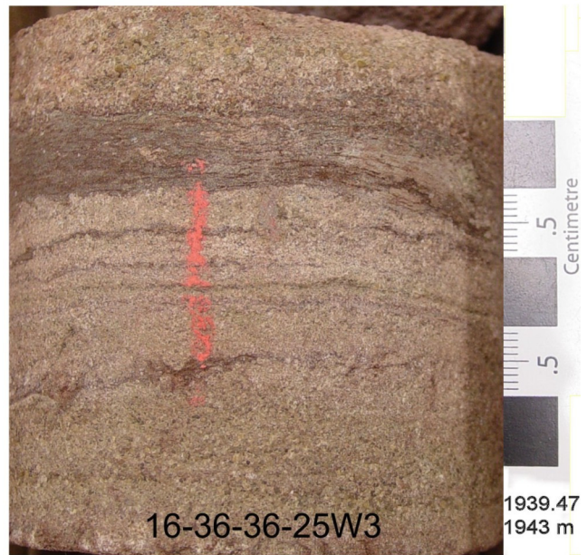
B. Mudstone laminae and thin beds interbedded with sandstone
