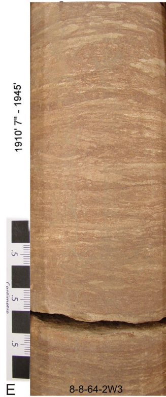
Very thin interbeds of sandstone and mudstone with some burrow structures.
