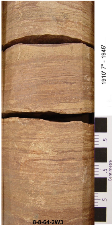
Very thin interbeds of sandstone and mudstone with some burrow structures.
