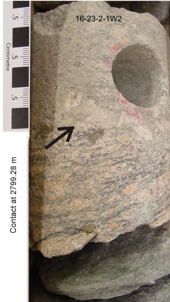
B. Contact at 2799.28 m between granite-pebble conglomerate and sandstone
