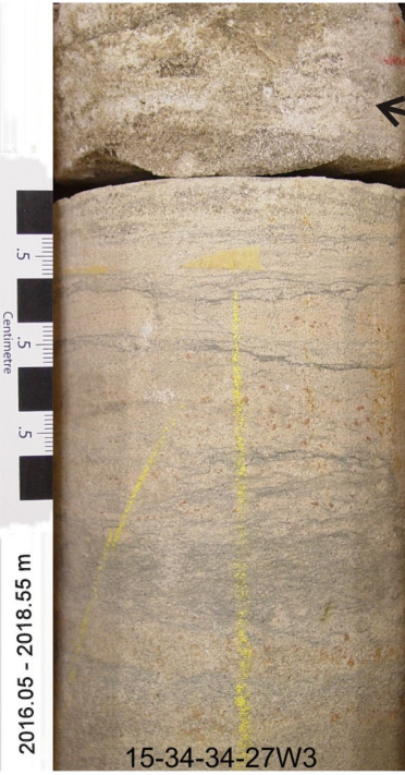
B. Bedded and bioturbated sandstone overlain by coarse-grained sandstone (arrow)
