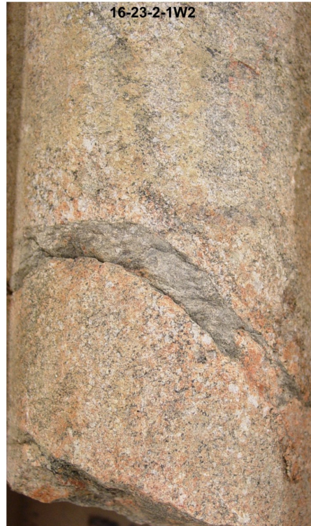
D. Granite basement with clay-filled fractures below 2800.78 m
