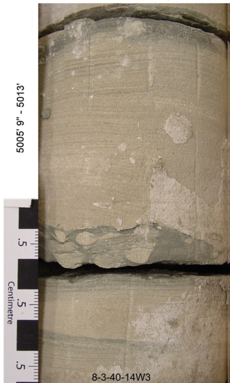
C. Sandstone with burrowed interbeds of mudstone
