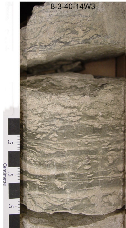
D. Core 13: extensively burrowed mudstone and sandstone
