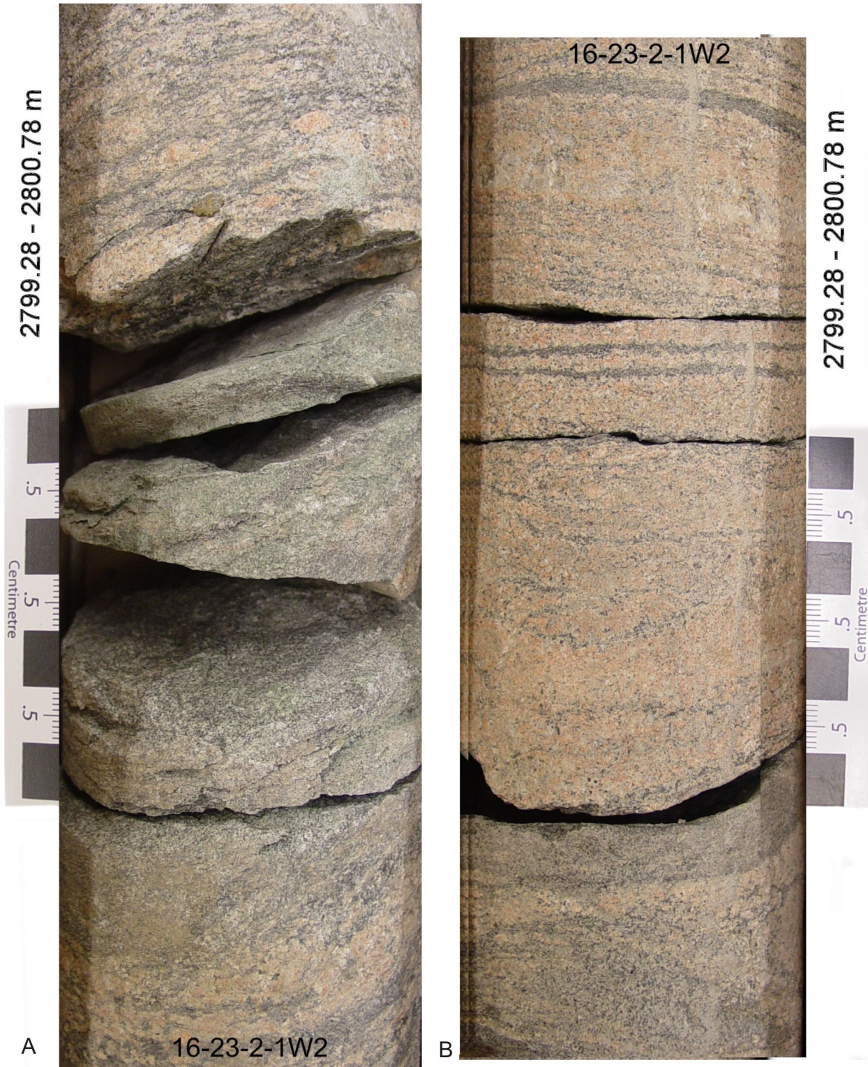
Examples of basal sandstone with varying amounts of basement-derived detritus
