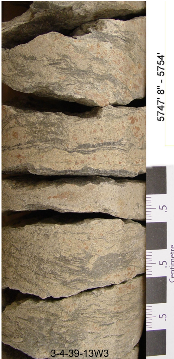
Extensively burrowed sandstone and mudstone
