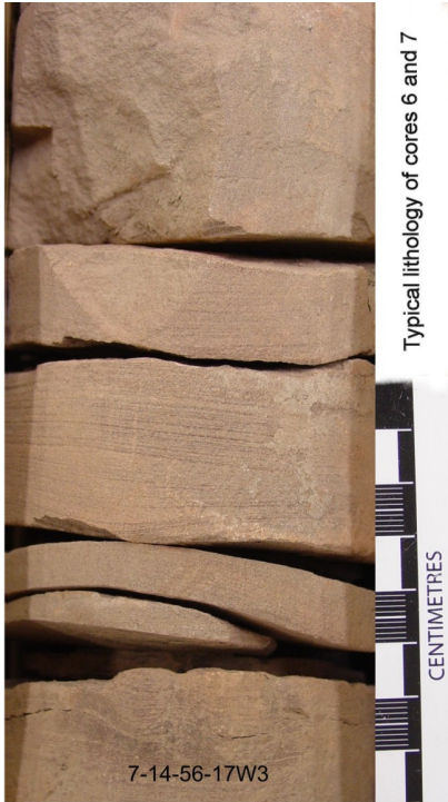
A. Typical facies of cores 6 and 7: red shale with fine laminae of sand/silt
