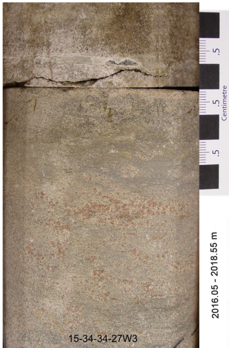
C. Interbeds of bedded sandstone and burrowed sandstone
