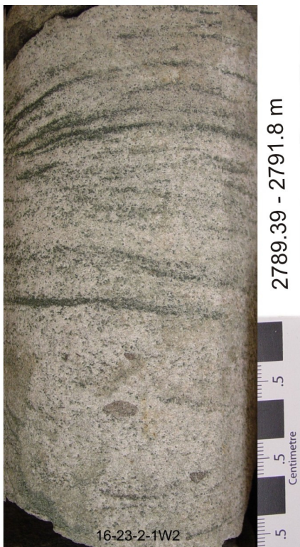
B. Cross bedded coarse-grained to granular sandstone
