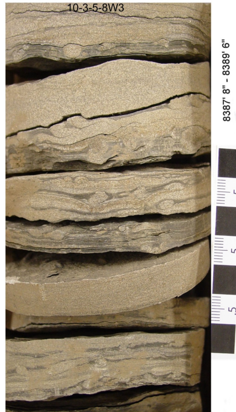
B. Thin interbeds of laminated and burrowed sandstone
