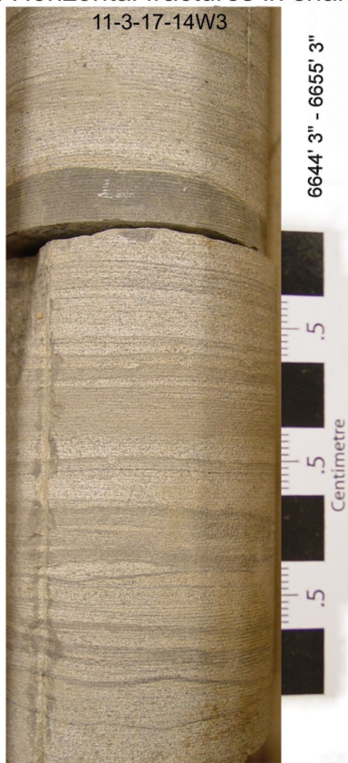
C. Horizontal and ripple laminated sandstone
