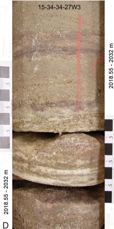
Cross bedded medium to granular sandstone
