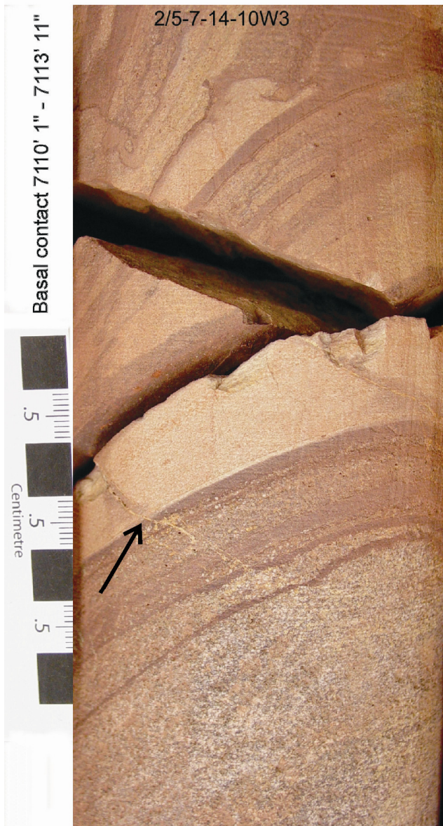
A. Contact between interbedded sandstone-limestone and arkosic sandstone at 7113' 11" (arrow). Over-steepened bedding
