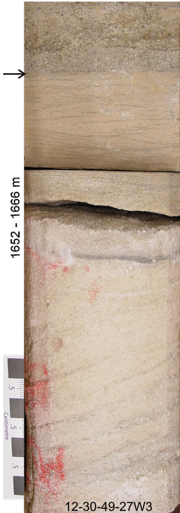
A. Fining-up bed: cross bedded medium to coarse-grained sandstone grading up into a mud-laminated fine grained sandstone, in turn erosionally overlain (arrow) by a coarse-grained sandstone
