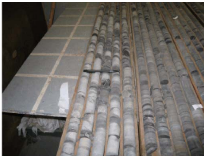
Figure 9. Limestone rich interval (pale shaded interval in the core) that marks the transition with the Trenton Group Six samples were collected from this core and analyzed
