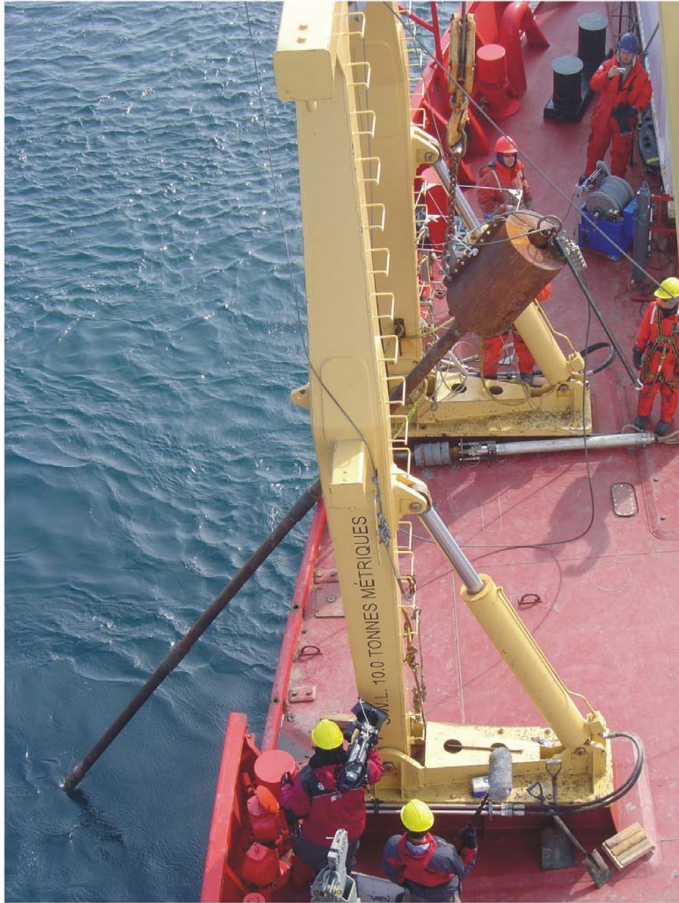
Figure 3.2: Piston corer deployment (Image courtesy T. Juul-Petersen)
