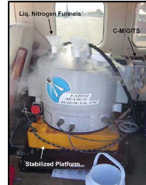
Figure 2. PROBE Hyperspectral Sensor.
