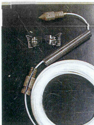
Figure 3: Waterloo Profiler tip connected to 1/4 inch polyethylene tubing shown with section of AW rod and coupler.
