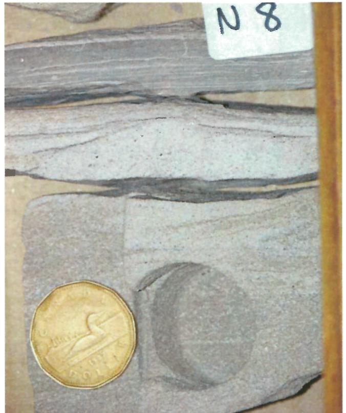
Photo 8: Parallel laminated, fine-grained sandstone and mudstone with siltstone laminae. Sparse or no bioturbation. Unit 3.
