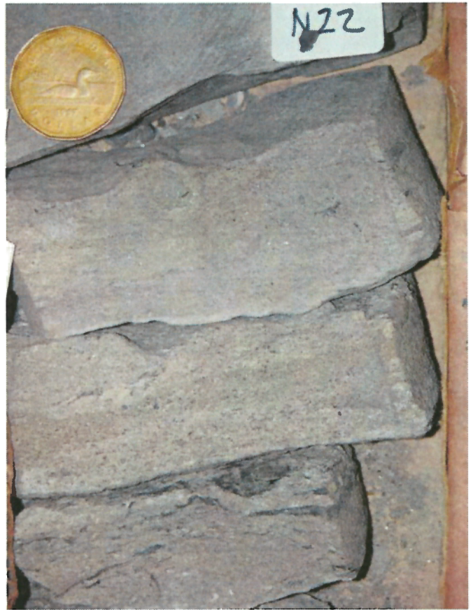
Photo 22: Fine-grained sandstone abruptly overlying coarse-grained sandstone, overlying medium-grained sandstone with large phytodetritus. Unit 12.
