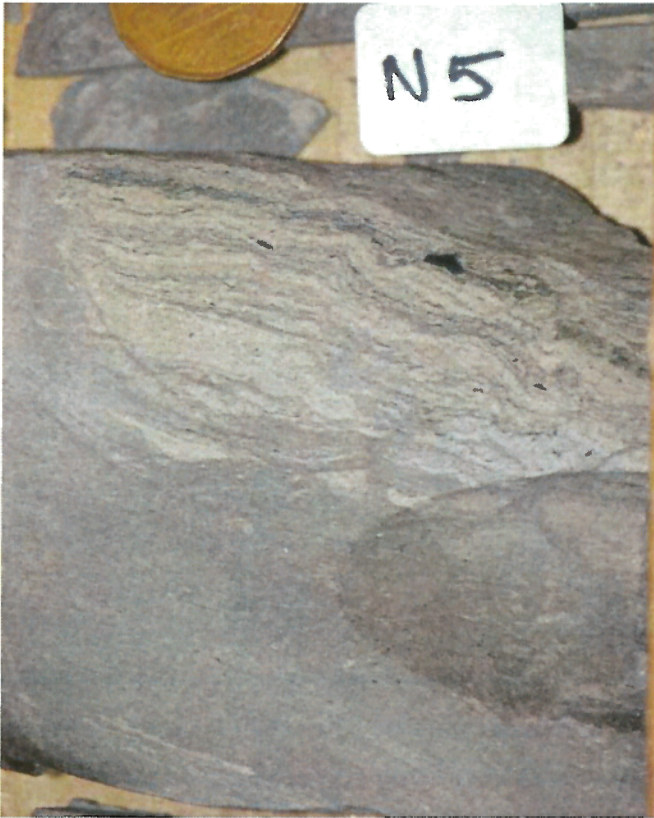
Photo 5: Deformed, fine-grained sandstone with lamina of phytodetritus at top, over dark silty mudstone. Unit 2.
