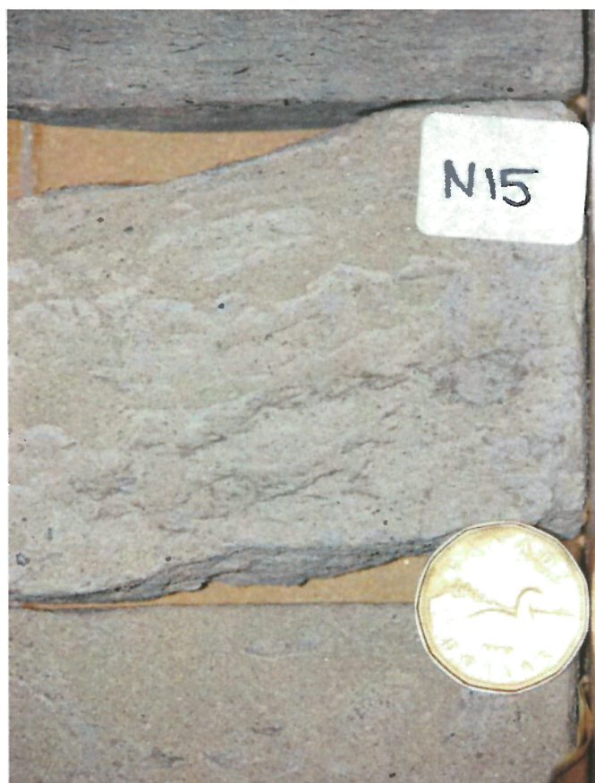
Photo 15: Fine-grained sandstone with mud drapes and mud-lined burrows. Below photo, overlies medium-grained sandstone. Unit 7.
