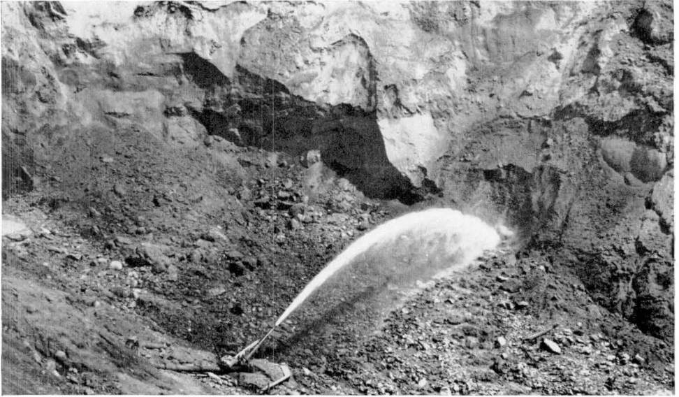
Hydraulic placer mining on Keithley Creek in the Cariboo district of British Columbia. Photo by A. H. Lang, Geological Survey (79974).
