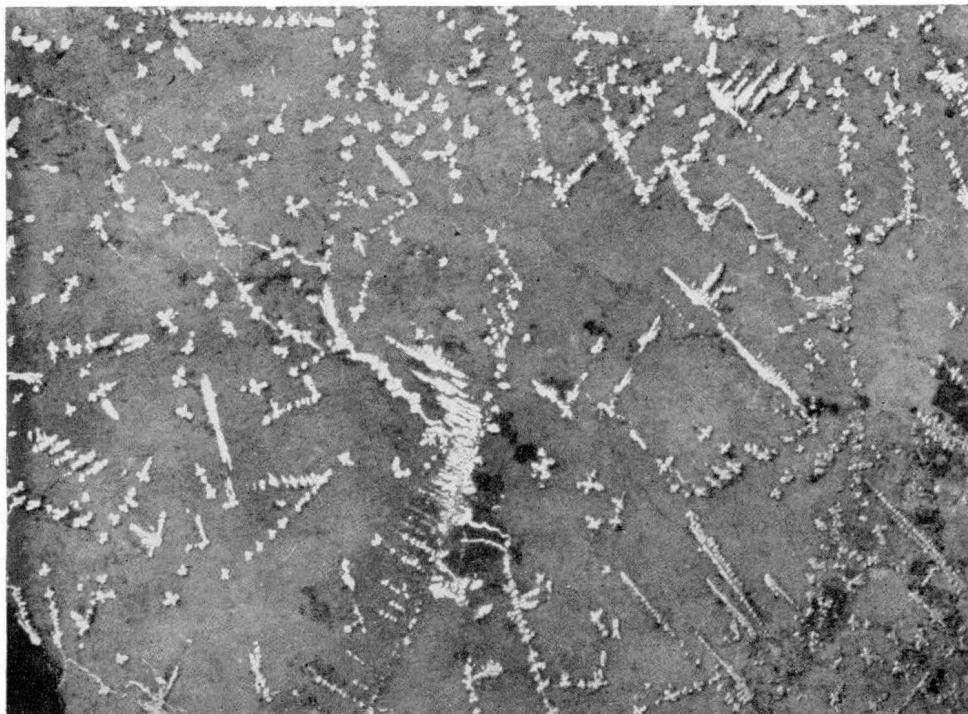
Native silver (white) in calcite, Temiskaming mine, Cobalt, Ontario, scale, about natural size. After Willet G. Miller, Ontario Bureau of Mines Report, 1913 (95917).
