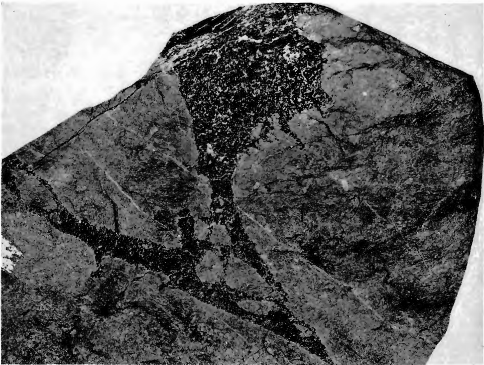
Specimen of dunite with chromite (black) filling fractures, Black Lake area, Quebec. Photo by Bureau of Geology and Topography; scale, \frac{1}{2} natural size (92167).
