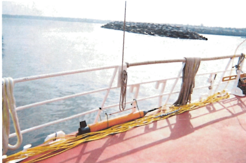
Figure 10- Setup of magnetometer while on deck.
