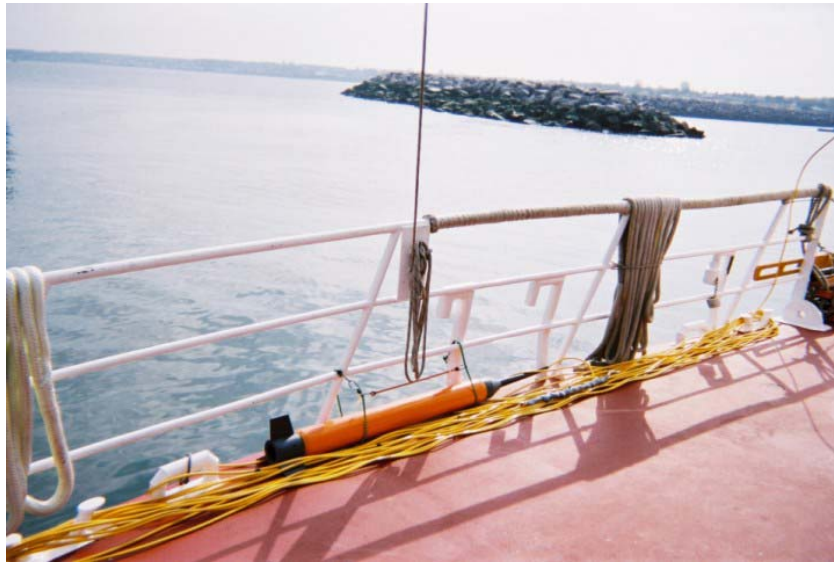
Figure 10- Setup of magnetometer while on deck.
