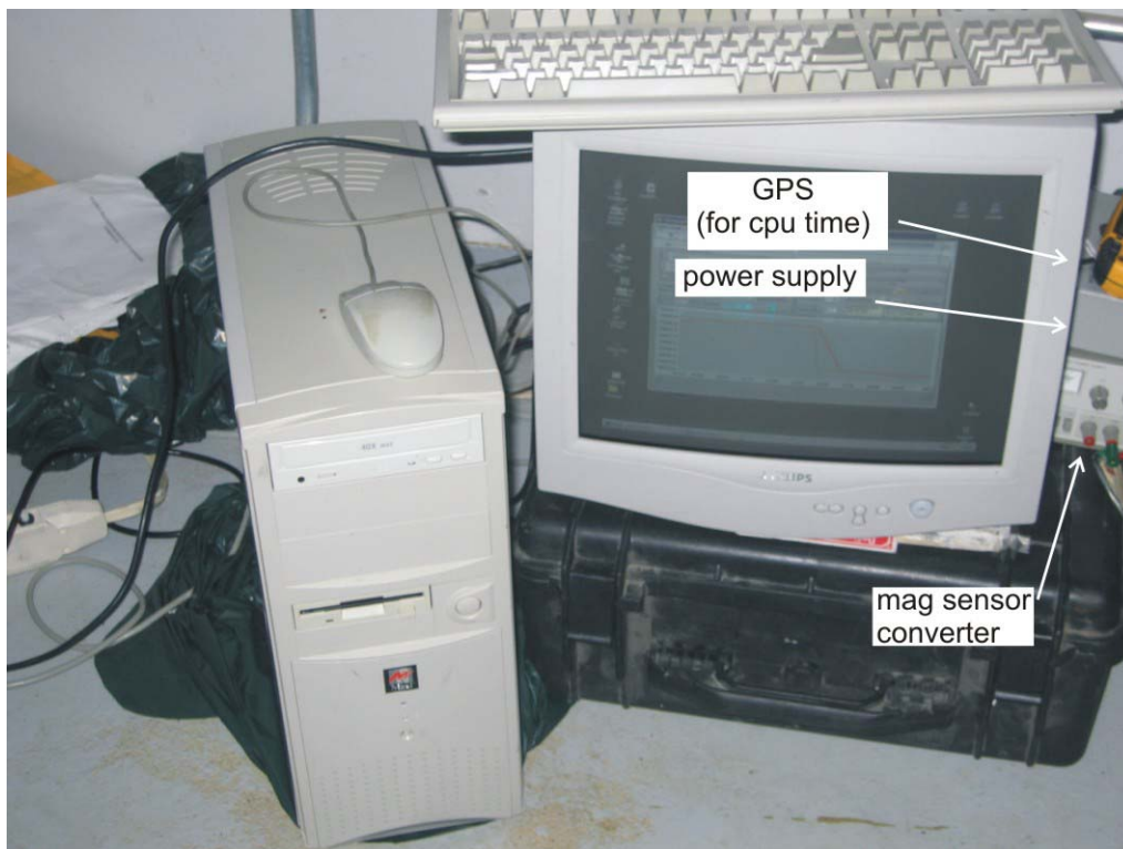
Figure 16- Station mag setup inside pump house.
