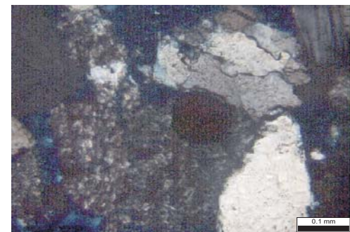
2212.20 m (pos. 2): quartz mylonite (weak) upper right mudstone intraclast (lower left) 200x xpl
