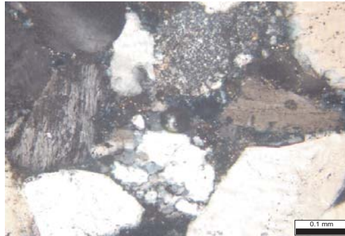
2211.47 m (pos. 4): microgranite (upper centre), quartz mylonite (weak) ( lower centre) 200x xpl
