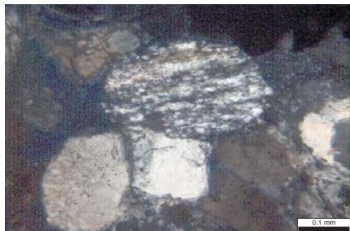
2212.20 m (pos. 1): microgranite/intrusive rhyolite (G), looks very similar to 2225.45 position 10. 200x xpl
