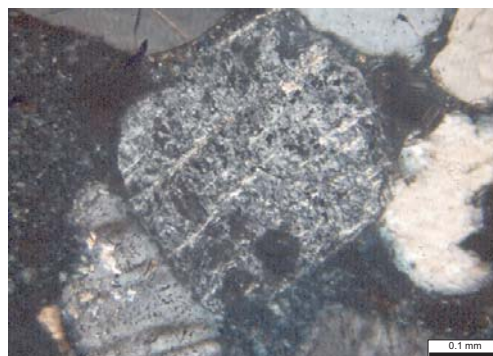
2230.62B m (pos. 5): Plagioclase crystal with inclusions of muscovite, and ferromagnesian minerals altering to siderite, probably from a granodiorite (EMP). 200x xpl
