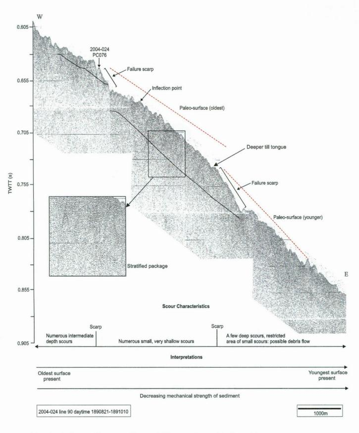
Transect A, figure c: Huntec profile on middle slope. Located in figure (a).
