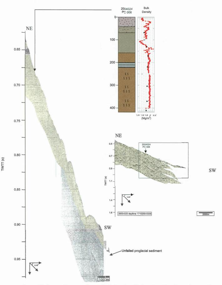
Transect K, figure a: Huntec profile near limit of surface till. Inset shows location on airgun profile.
