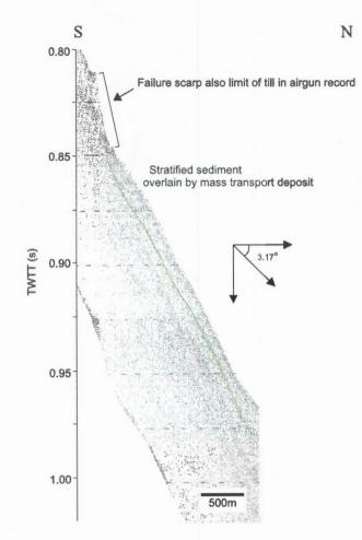
Transect C, figure c: Huntec profile showing limit of till body imaged in figure (a).
