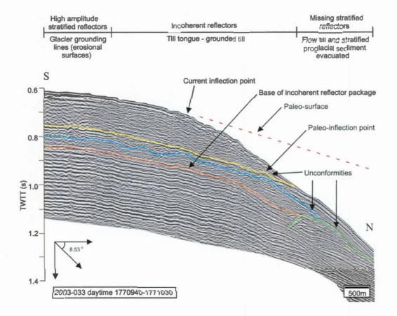
Transect D, figure a: Airgun profile showing aggradation of till on outer shelf.
