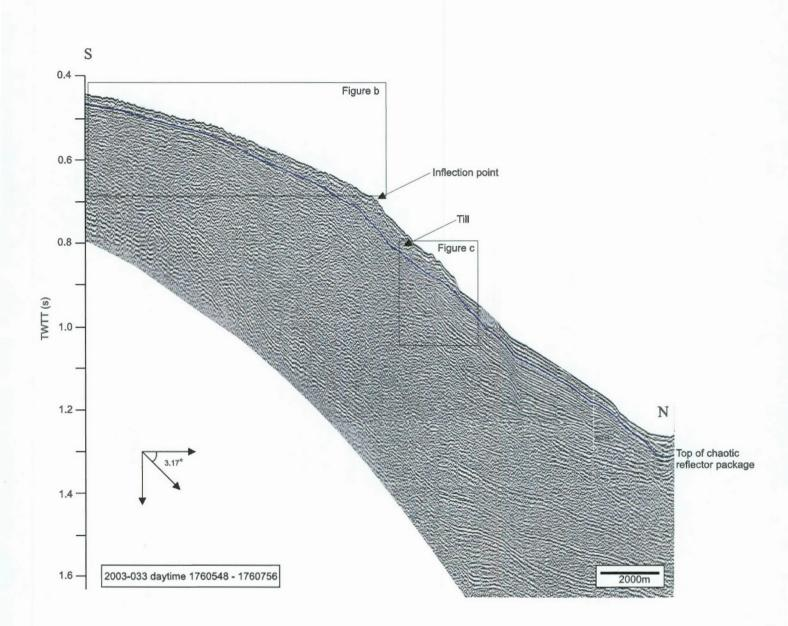
Transect C, figure a: Airgun profile showing pinch-out of till above blue horizon.
