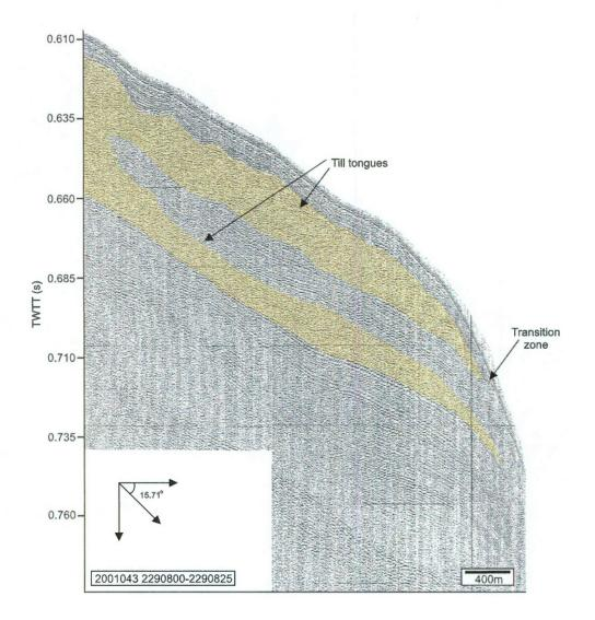
Transect O, figure a: Huntec profile showing stacked upper slope till tongues, Stratigraphy for Piper et al. (2005) and McCall (2006).
