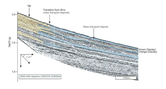
Transect V, figure a: Airgun profile showing transition from upper slopt till to mass-transport deposits.
