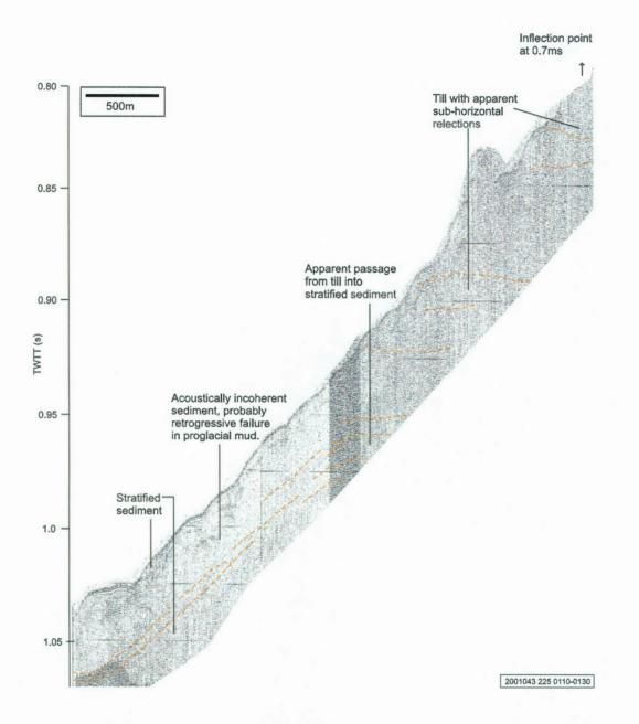
Transect O, figure b: Huntec profile showing highly reflective till outcropping below inflection point and passing into stratified sediment with retrogressive failure.
