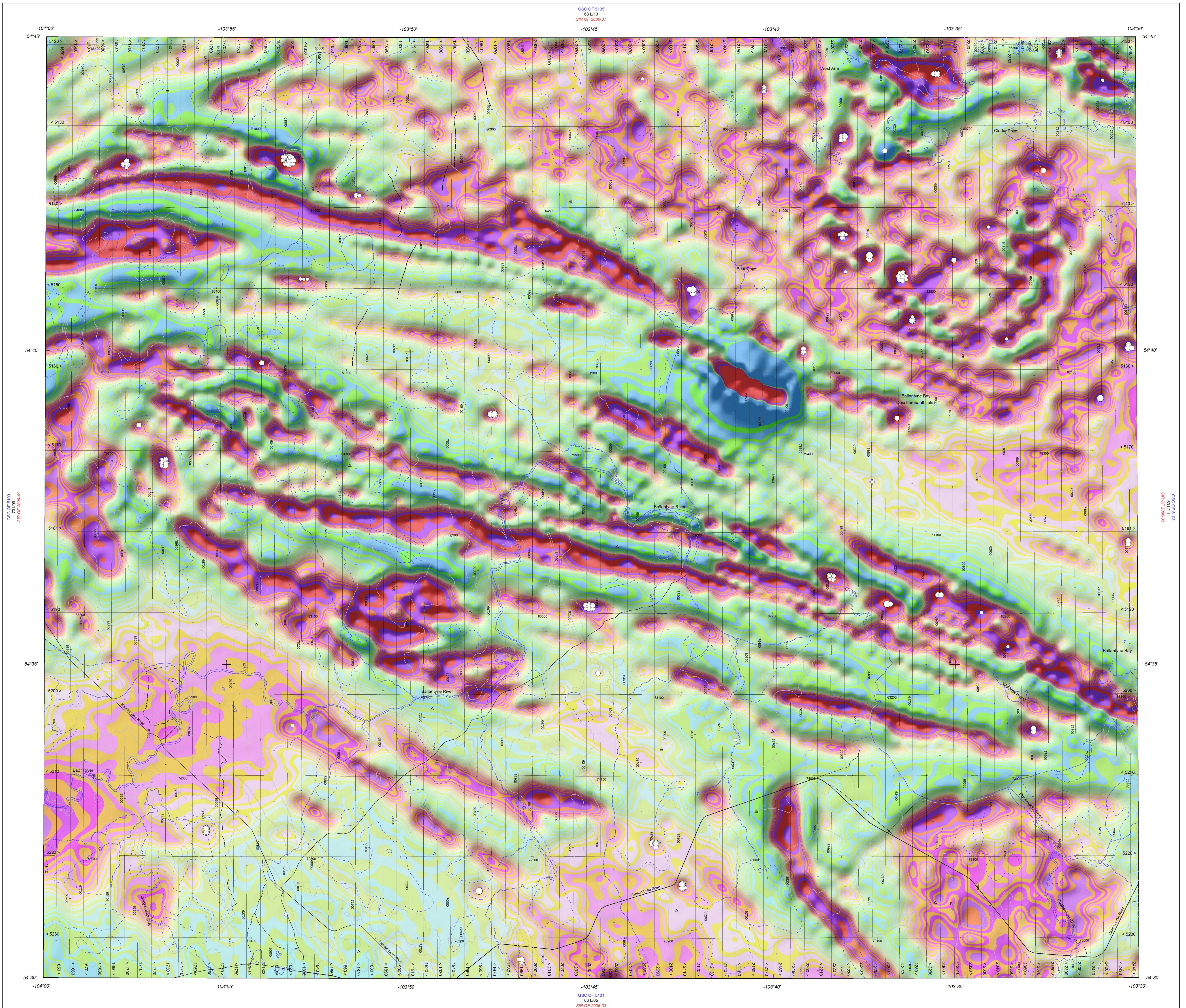
This map was compiled from data obtained as a result of an aeromagnetic survey carried out by Fugro Airborne Survey using a Cessna Caravan registration C-FZLK aircraft. A 1.000 m NT sensitivity split-beam cesium vapour magnetometer was mounted in the tail boom of the survey aircraft.
