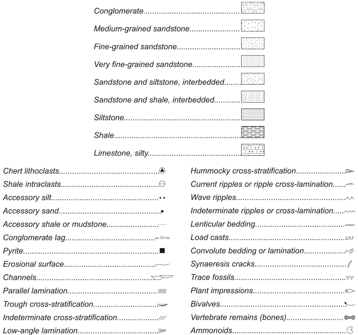
Figure 3: Legend of rock types, sedimentary features, and fossils to accompany measured section MWB-00-03 (Figure 4).
