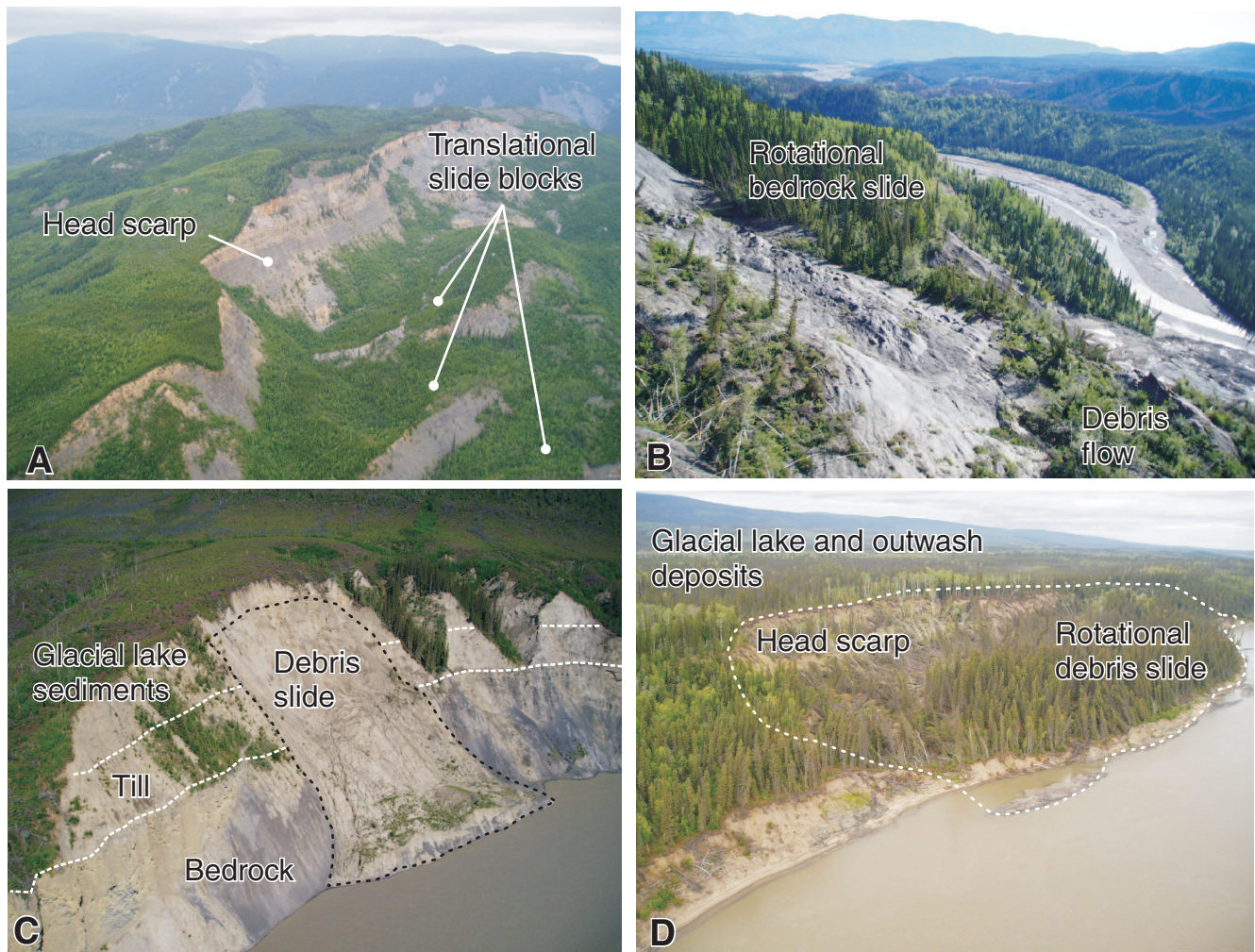
Figure 3. A) Camsell Range, Mackenzie Mountains: translational slide in shale, sandstone, and carbonate triggered by postglacial uplift, gravitational spreading, and valley incision. B) English Chief River, Mackenzie Lowland: rotational slide in weak shale and carbonate triggered by rapid postglacial incision by river; note that colluvial shale and glacial debris are remobilized as secondary debris flows. C) Redstone River, Mackenzie Lowland: rapid planar debris slide triggered by melting of discontinuous permafrost in glaciolacustrine deposits and till exposed by cutbank erosion (evolving into debris flow). D) Mackenzie River, Great Slave Plain: rotational debris slide involving till, glaciolacustrine deposits, and glaciofluvial outwash triggered by cutbank erosion.
