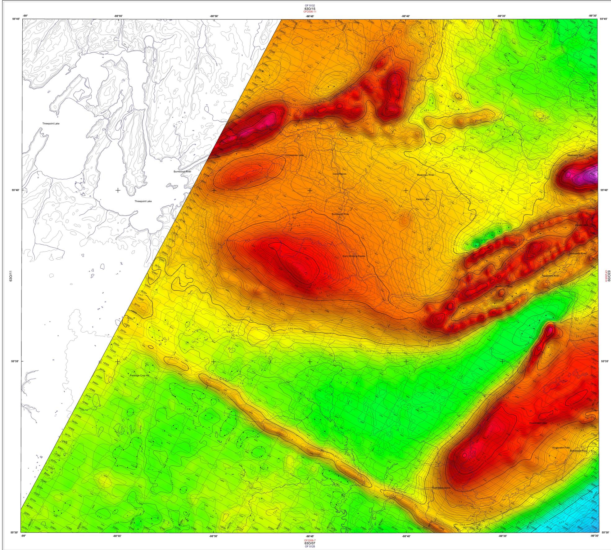
This map was compiled from data obtained as a result of an aeromagnetic survey carried out by Goldak Airborne Surveys using a Piper Navajo (registration C-GJBB) aircraft. A 0.005 nT sensitivity split-beam cesium vapour magnetometer was mounted in the tail boom of the survey aircraft.
