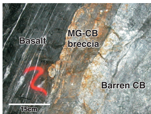
Figure 7. Carbonate-magnetite breccia showing clasts of iron carbonate vein in a magnetite-rich matrix developed along the wall of a barren iron-carbonate vein, section view (CB - carbonate, MG - magnetite).
