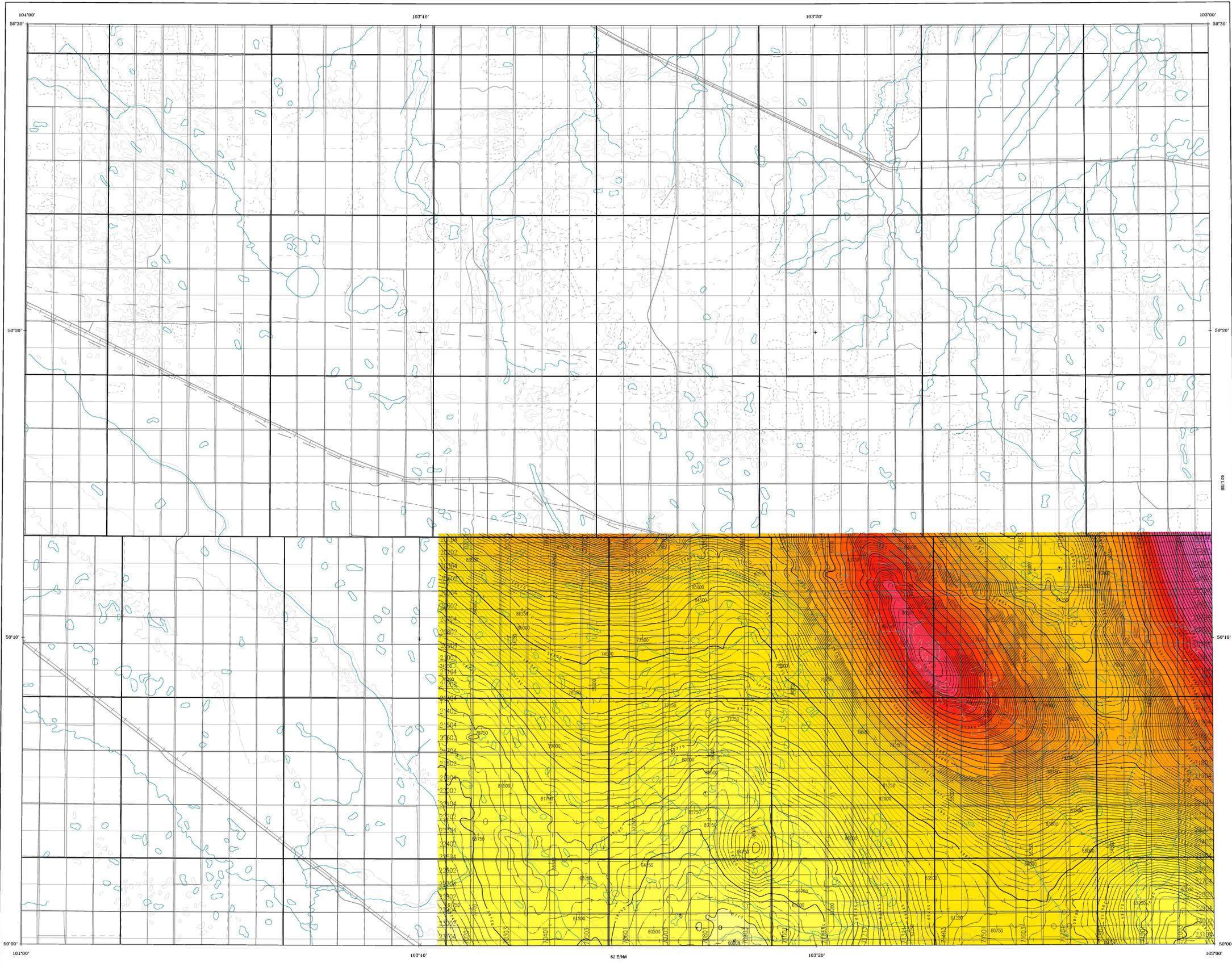
This map was compiled from data obtained as a result of an aeromagnetic survey carried out by SIAL Géosciences Inc. using a NAVAJ0 310 aircraft (registration C-FYTT). The survey was funded by Wascana Energy Ltd. and monitored by the Geological Survey of Canada. A 0.005 nT sensitivity split-beam cesium vapour magnetometer was mounted in the ballroom of the survey aircraft.
