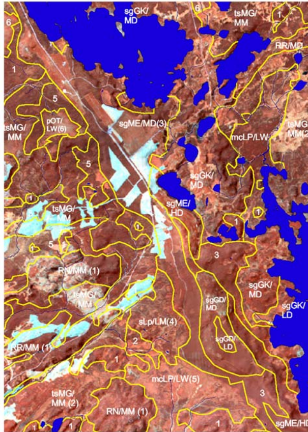
Figure 4. A subarea of the Landsat 4-5-7/DEM merged image shown in Figures 2 and 3 (boundaries are outlined in Figure 3B) displaying engineering terrain units interpreted from remotely sensed imagery, the DEM and DEM derivatives. Terrain unit classification is based on four components: materials, landform, relief and moisture. As an example, the unit classified as sgME/MD (labelled above as (3)) has four components; sg indicates that it is composed of the materials sand and gravel; ME indicates that the landform it comprises is an end moraine; M (following the slash) indicates that the relief is moderate; and D indicates that moisture conditions are dry. A key is provided below.
