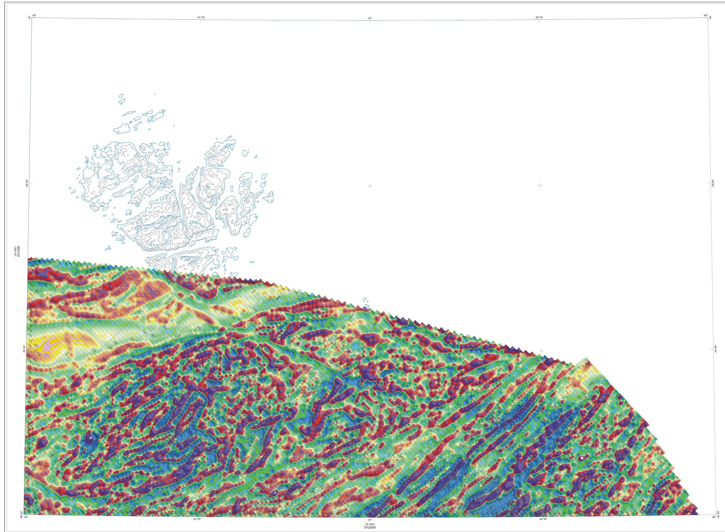
This map was compiled from data obtained as a result of an aeromagnetic survey carried out by FUGRO Airborne Surveys using a Cessna C-206 Caravan (registration C-FZLK) aircraft and a Cessna C-404 (registration C-FYAU) aircraft. A 0.005 nT sensitivity split-beam cesium vapour magnetometer was mounted in the tail boom of the survey aircraft.
