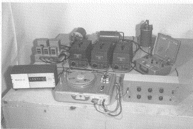
This instrument, used by Bancroft in the Lake Superior project, records the output of three seismometers on FM magnetic tape. It is a far cry from the cumbersome equipment used in the rockburst work!
