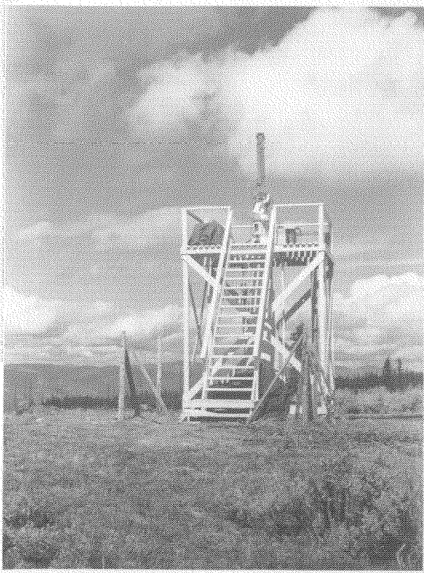
Observing platform, telescope and ciné camera used by Gaizauskas to monitor daytime seeing on Mount Kobau.
