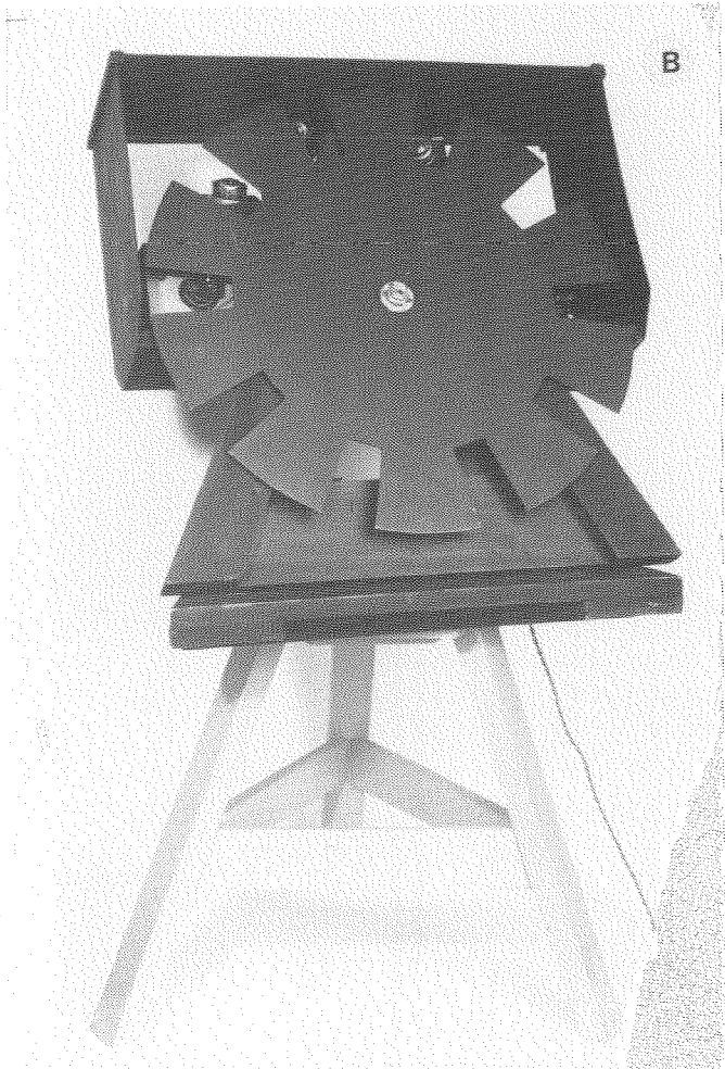
Left, 1937 version of camera and recording shutter and, Above, a more advanced, 1946 version. The 1946 system has five cameras, two spectrographic and three direct, behind a large rotating shutter.
