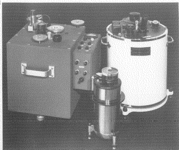
Early gravimeters. From the left: Atlas, Worden, North American.
