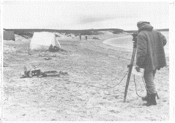
Observing with the portable fluxgate magnetometer.
