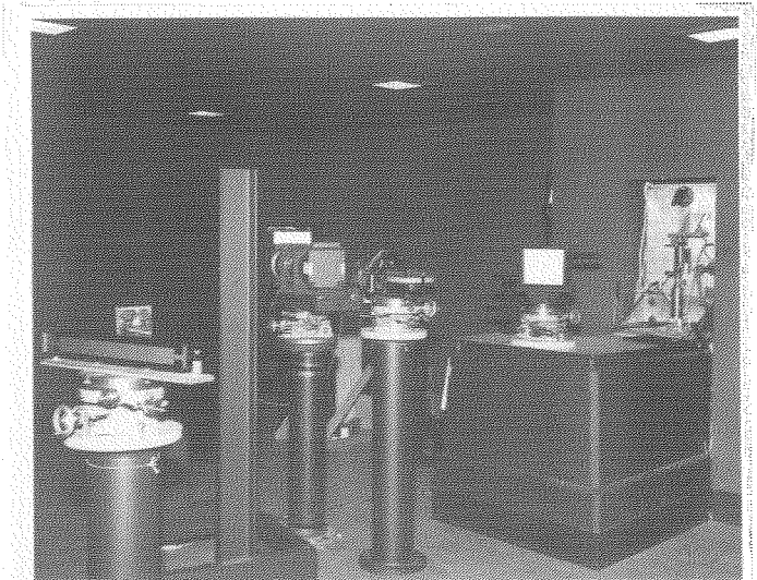
Partial view of the coudé spectrograph of the 48-inch telescope. The slit is in the wooden panel to the right; the bright rectangular patch to its left is the grating for the short focal-length camera. The pillars and girder support the camera mirrors and plate holders.
