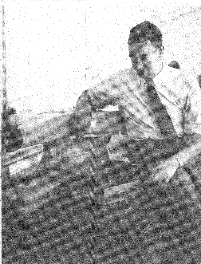
J.E. Kennedy with the Hilger ultraviolet prism spectrograph used in the airborne expedition to study the eclipse of June 30, 1954.
