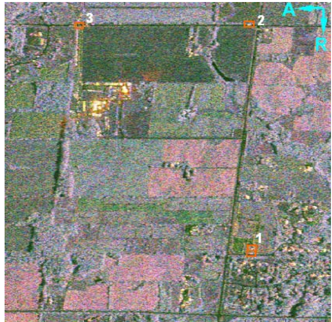
Figure 1. Ground-processed C-SAR colour imagery of pipeline right-of-way area on September 29, 2001 (Red:HH, Green:VV, Blue:HV). Arrows indicate range (R) and azimuth (A) directions. Orange rectangles indicate the vehicle locations.
