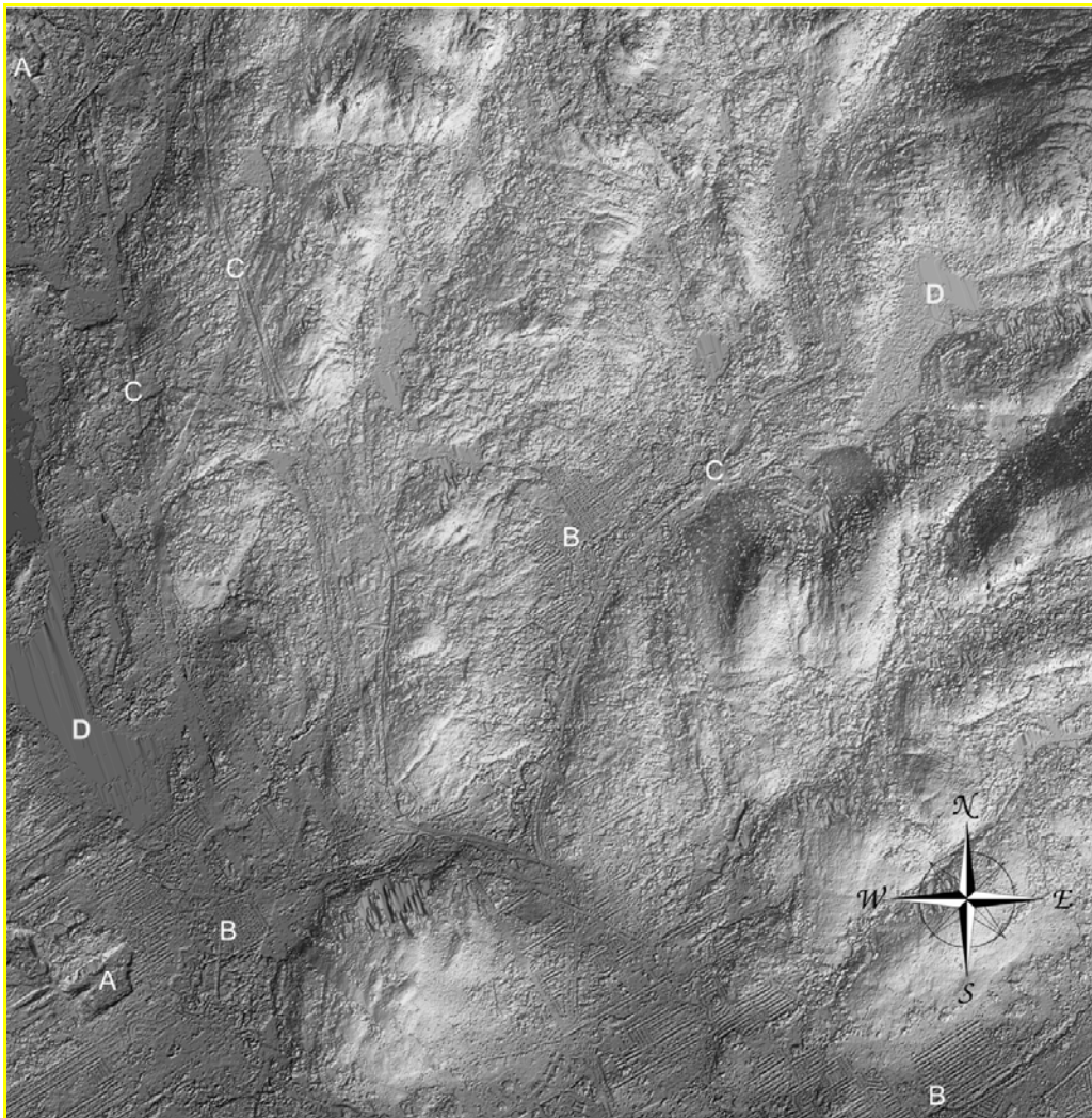
Figure 9. DEM (10 km × 10 km; 1 m spacing) extracted from the IKONOS-II stereo-pair. Noticeable cartographic features include: (A) sand pits, (B) residential areas, (C) roads and power lines, and (D) lakes. The linear features, which occur in residential areas (B), are not artefacts or systematic errors but are related to streets and houses patterns.
