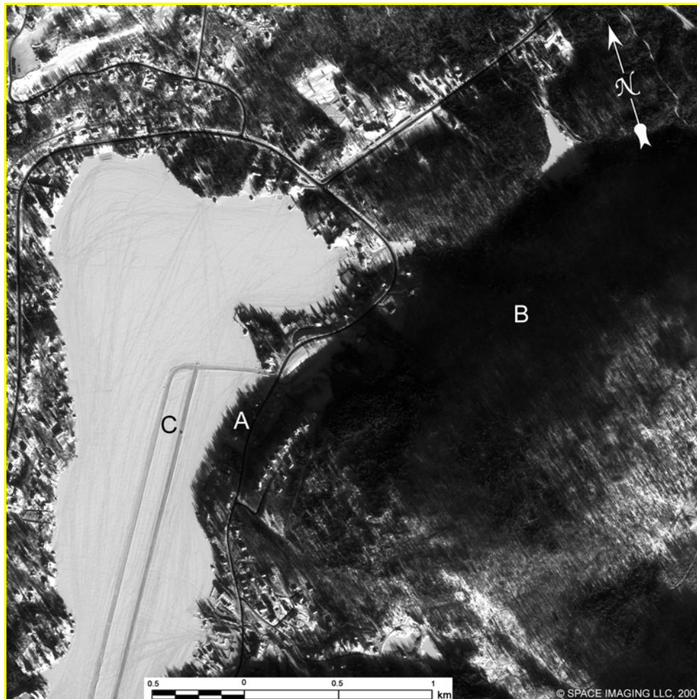
Figure 3. Subimage of backward image of the IKONOS-II stereo pair, north of Québec City, Québec, Canada. Note (A) tree shadows, (B) mountain shadows due to 19^\circ solar elevation angle and 166^\circ azimuth angle, and (C) a skater on the frozen lake.
