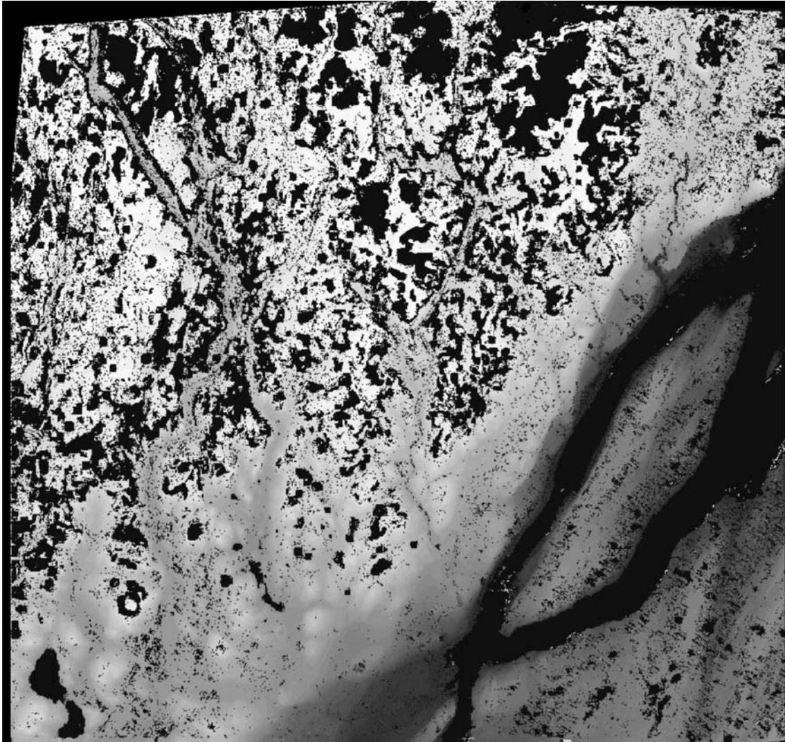
Figure 4. DEM (60 x 60 km; 5 m spacing) extracted from the two SPOT-5 stereo pairs. The black areas correspond to matching errors generated from radiometric differences between the multirate images: due to melting snow in the mountains, frozen lakes and the St Lawrence River (see Fig. 1).
