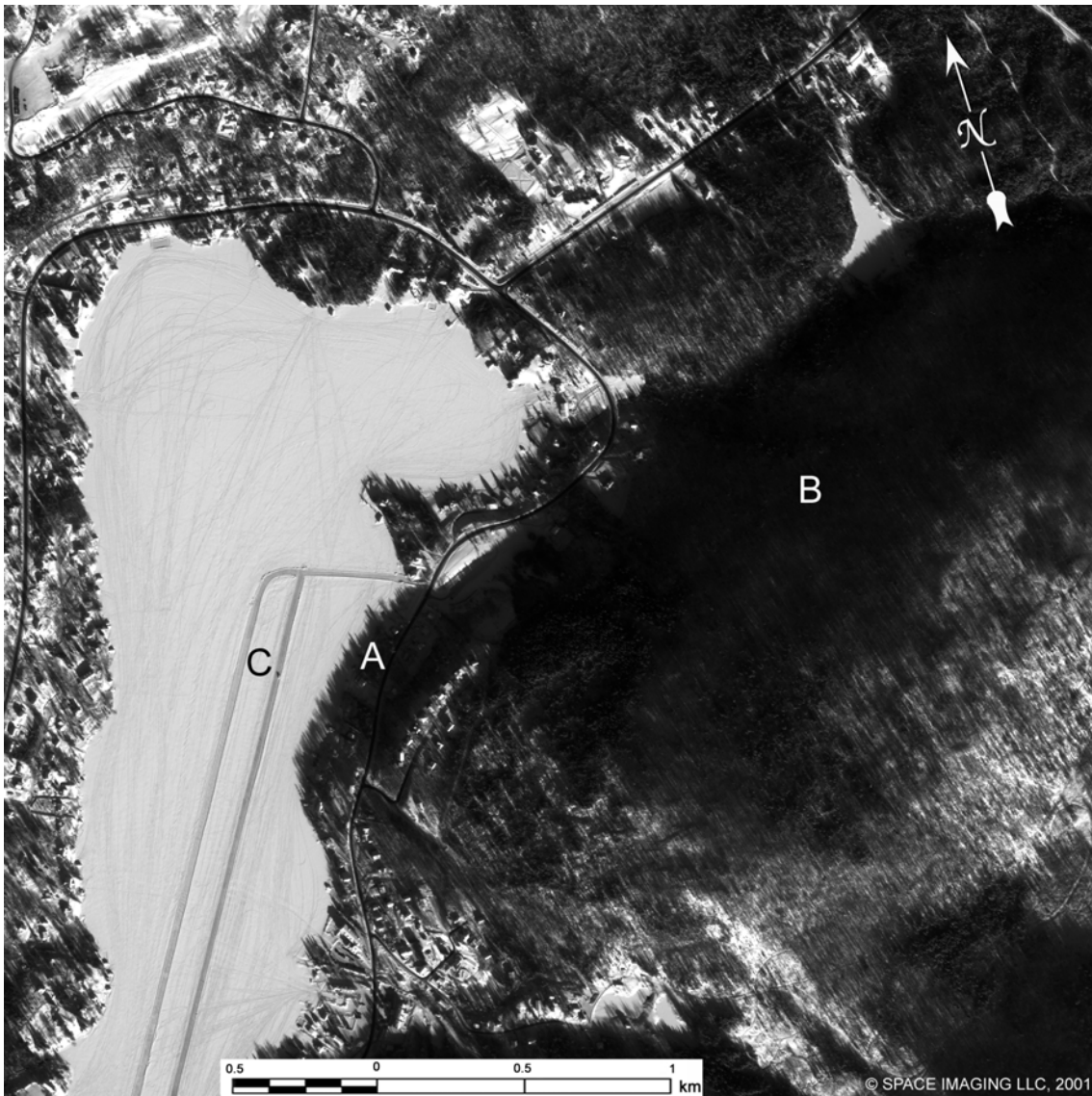
Figure 2. Sub-image of backward image of the IKONOS stereo pair, north of Québec City, Quebec, Canada. Note (A) tree shadows and (B) mountain shadows due to 19^\circ solar elevation angle and 166^\circ azimuth angle and (C) a skater on a frozen lake. IKONOS Image © Space Imaging LLC, 2001.
