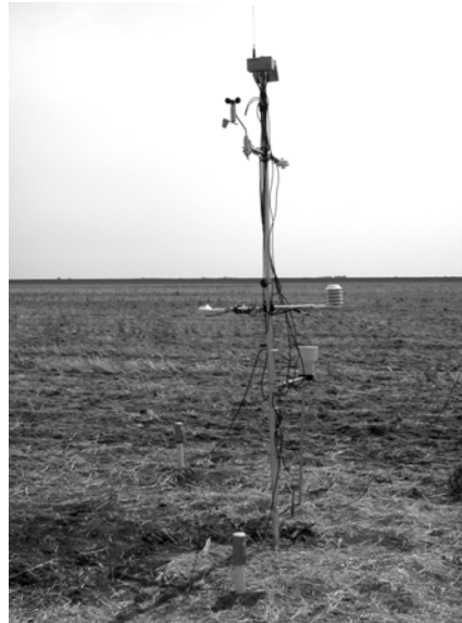
Figure 2. Adcon node 15263, with C-Probes 15262 and 18844 in the ground, deployed in the North Field at BLS.
